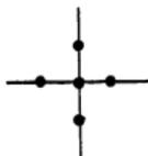
$$\begin{aligned}\nabla^2 u_{0,0} &= \left( \frac{\partial^2 u}{\partial x^2} + \frac{\partial^2 u}{\partial y^2} \right)_{0,0} \\ &= \frac{1}{h^2} (u_{1,0} + u_{0,1} + u_{-1,0} + u_{0,-1} - 4u_{0,0}) + O(h^2)\end{aligned}$$
