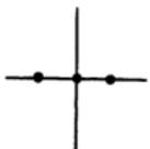
$$\frac{\partial^2 f_{0,0}}{\partial x^2} = \frac{1}{h^2} (f_{1,0} - 2f_{0,0} + f_{-1,0}) + O(h^2)$$
