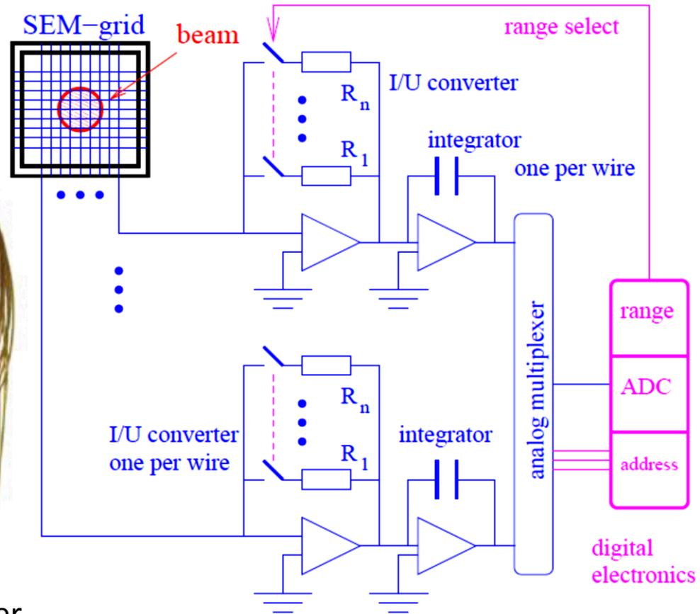
Each wire is equipped with one I/U converter
