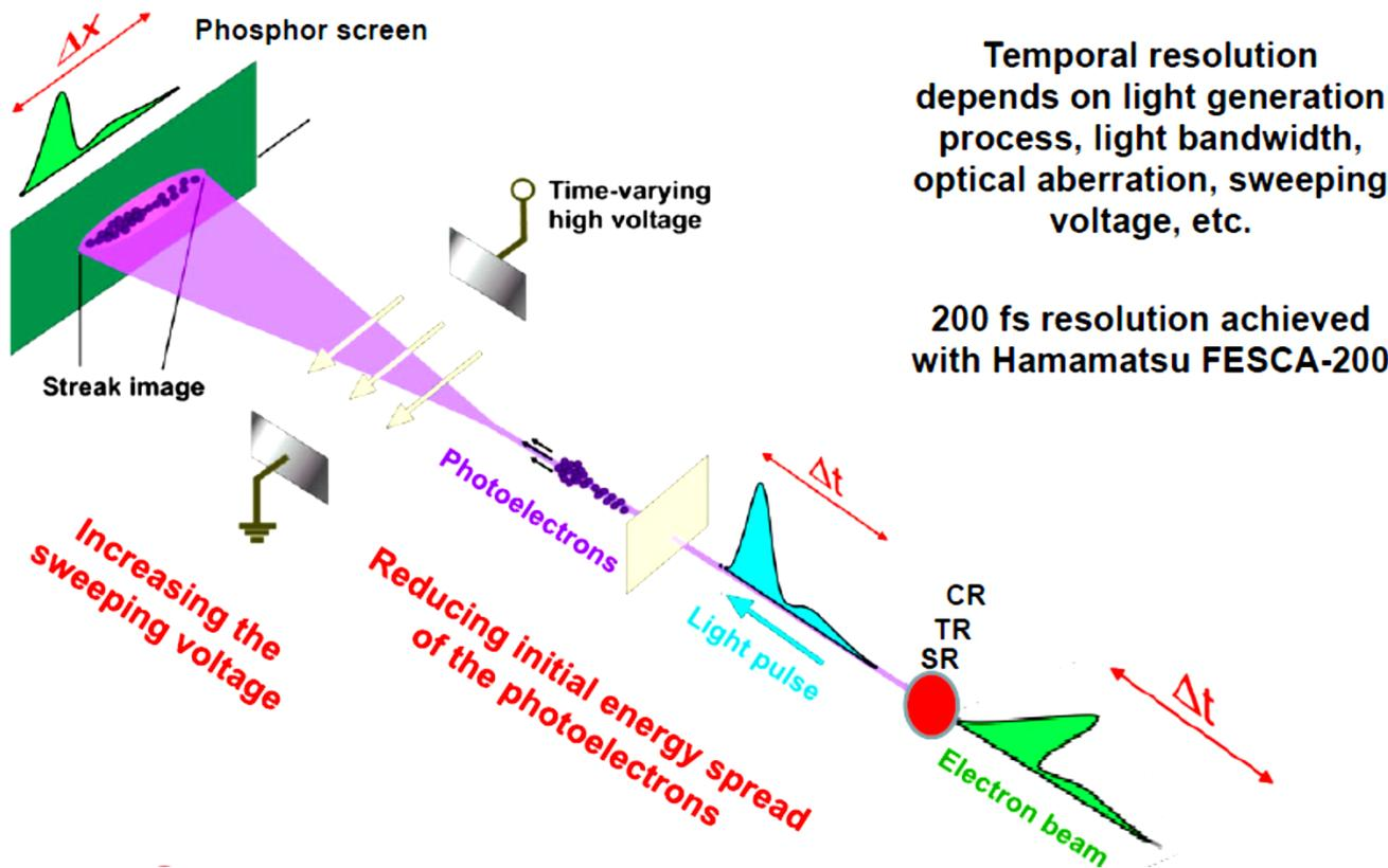
Temporal resolution depends on light generation process, light bandwidth, optical aberration, sweeping voltage, etc.
