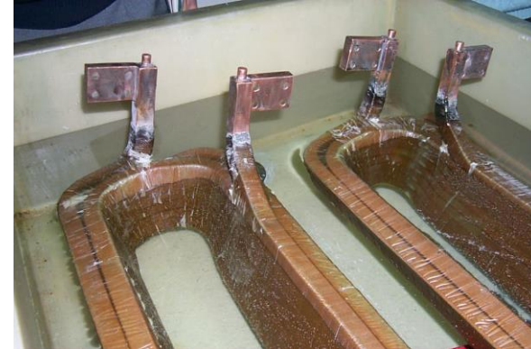
coil electrical test (under water !)
