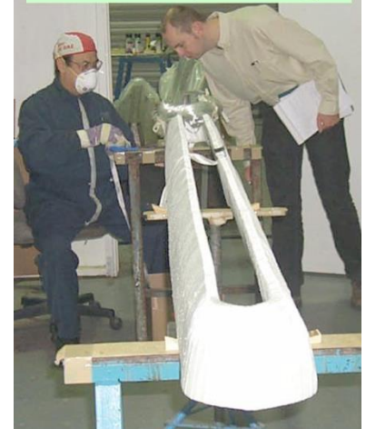
Glass fiber tape winding
