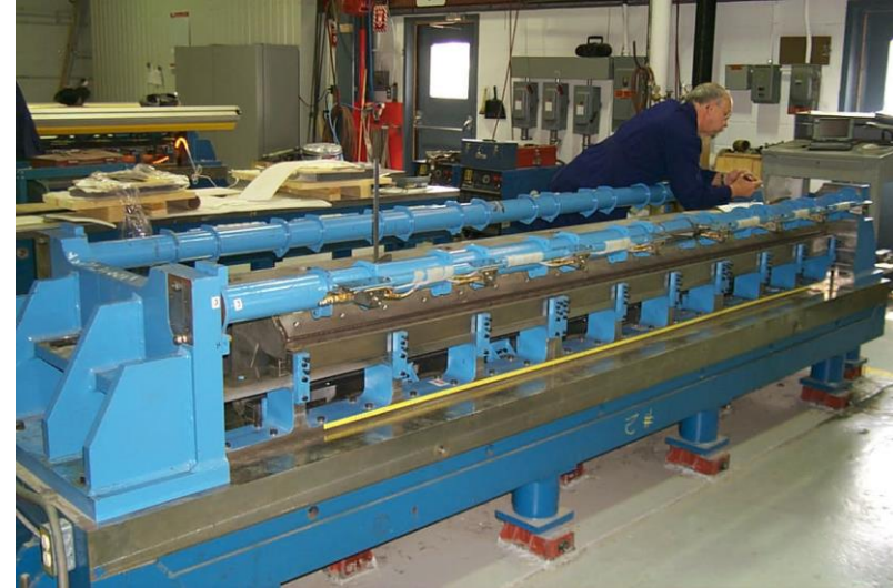
Stacking an MQW quadrupole yoke stack
