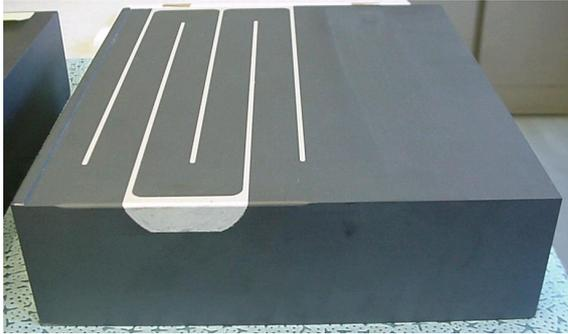
(a) A ferrite block with printed metallic stripes.
