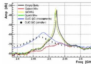
Resonant cavity signal in presence of Carbon (36 μm), Silicon Carbide and Quartz wires
