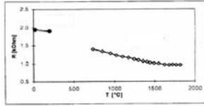
Fig 4: Measured wire resistance variations with temperature.
