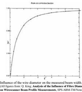
Influence of the wire diameter on the measured beam width.
