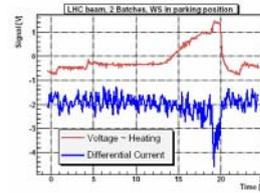
Wire heating due to the LHC beam injection in the SPS (No scan, wire in parking position). The beam energy ramp/bunch length decreasing begin t=11 s.
