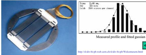
SEM grid with 15 foils to measure the beam profile. The large foils at either side of the grid are connected electrically together to form a 16-th channel.
