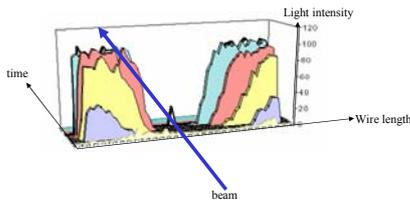
Digitized video recording of an 8 μm carbon wire scanning a 0.8 mA beam. The wire is parallel to the horizontal axis, and the light intensity is plotted along the vertical axis (arbitrary units). Successive profiles are separated by 20 ms. The central spot corresponds to the passage of the wire through the beam. Thus, RF heating led to (huge) thermal glowing before the beam interacts with the wire.
