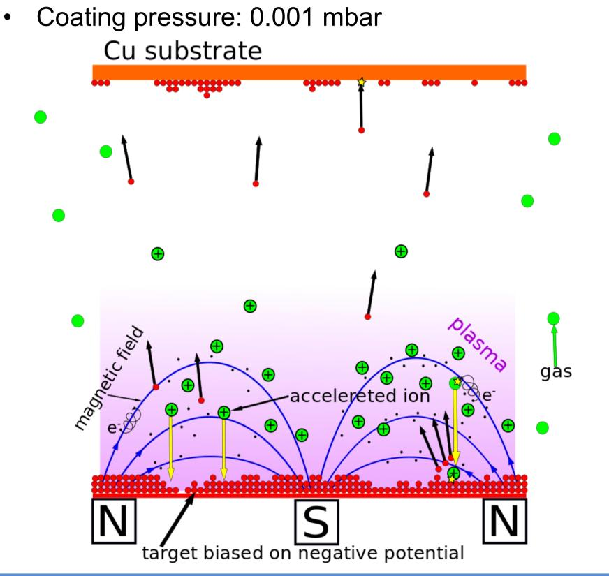
**Step1**: Sputter Ta on a Cu substrate **Step2**: Transform brittle Ta beta-phase into stable alpha-phase by annealing **Step3**: Coat Nb<sub>3</sub>Sn on top of Ta layer **Step4**: Annealing of Nb<sub>3</sub>Sn for A15 superconducting maintaining structure
