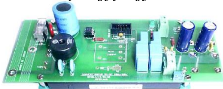
600 W, 300 V DC /30 V DC converter
