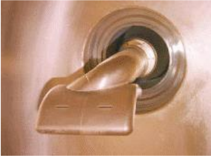
Capacitive coupler of CERN PS 40 MHz
