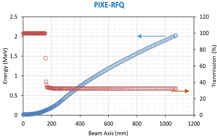
March 2019, proposition for the construction at CERN of a new PIXE-RFQ, which will produce a proton beam of 2 MeV which will be extracted in air.
