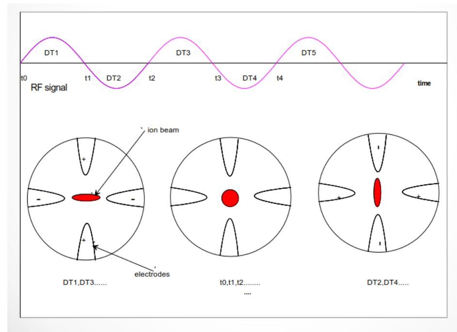
→ RF Field produces alternating gradient focusing (Electric Quadrupole)
