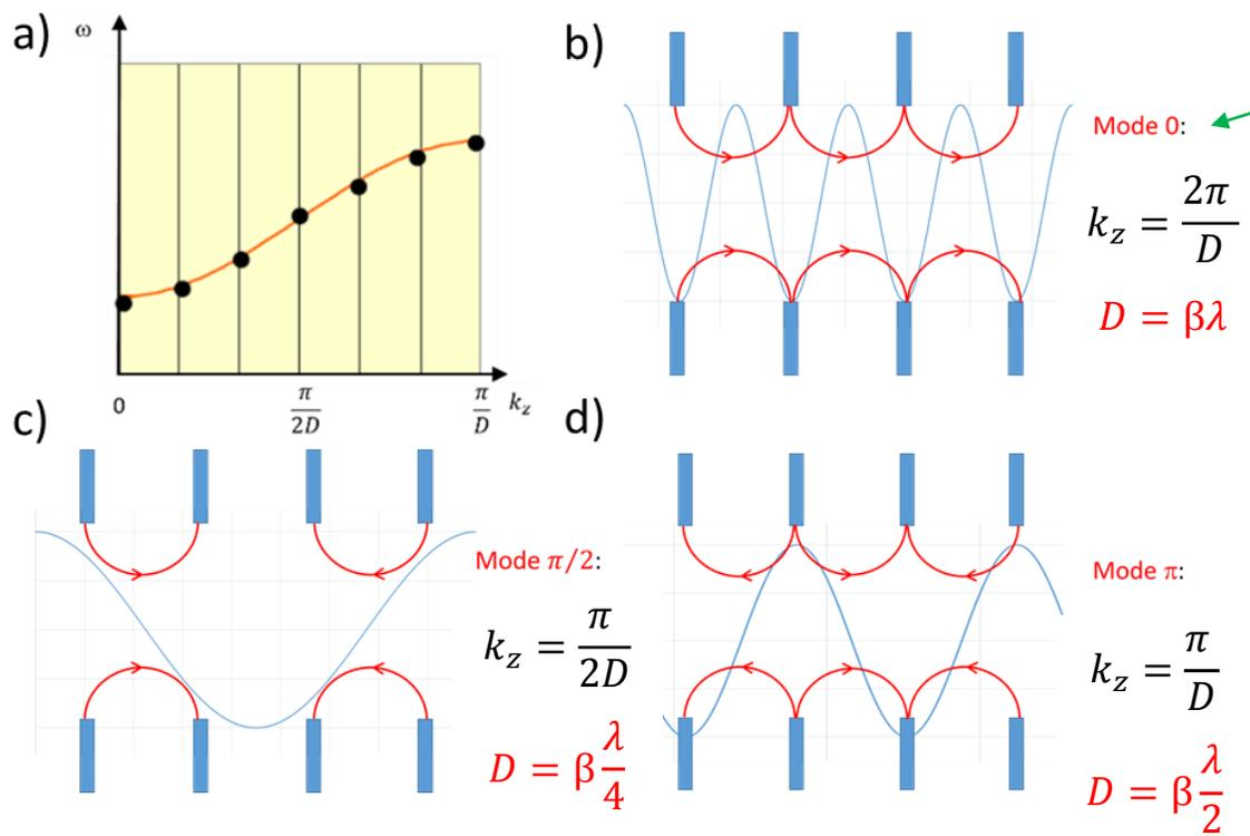
The DTL (Drift Tube Linac) is an example of “Mode 0” TM cavity
