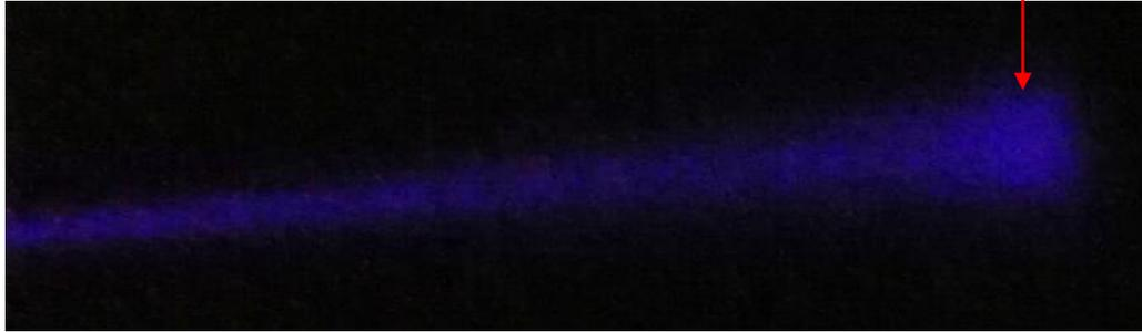
**Observation of the Bragg peak:** The beam is more visible at the end of the trajectory. This explains the advantages of the hadrontherapy!
