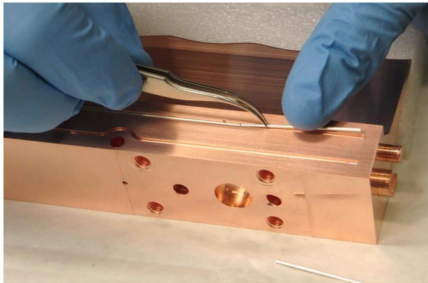
(Grooves on one side for the minor vanes and on the brazing surface of the top major vane)
