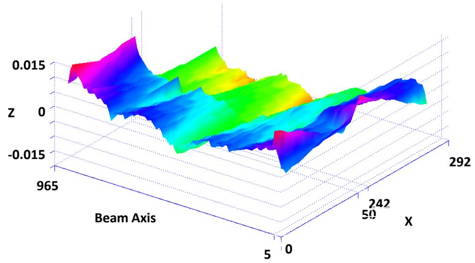
Geometry of the brazing planes after machining. Dimensions are in mm. The flatness is better than 10  $\mu\text{m}$  over one meter. (Note: This major vane has been rough machined and heat treated at 600 °C before final machining)
