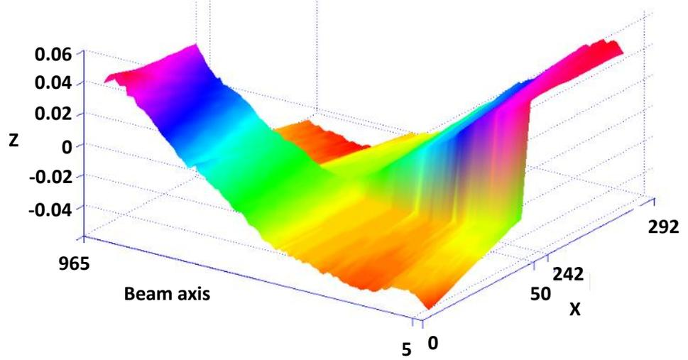
Geometry after a heat treatment at 800 °C. The deformation is more than 80  $\mu\text{m}$ , not acceptable for vacuum brazing! ( $\approx 20 \mu\text{m}$ )
