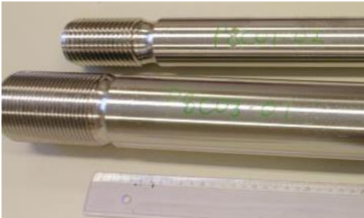
Inconel 718 for ITER magnet supports.
