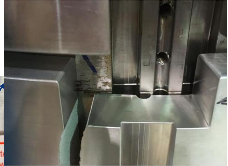
Catastrophic failure of MQXFAP2 Al shell. Failure analysis: EDMS 2088319
