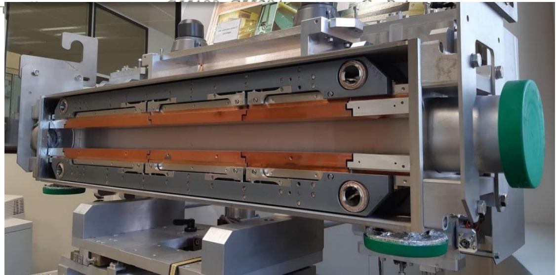
CERN Phase II collimator. Glidcop® sectorized jaw
