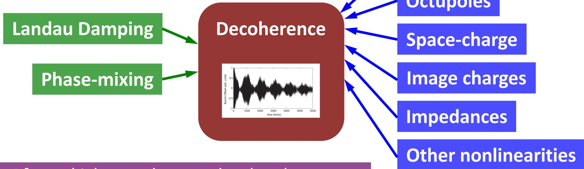
After a kick, we observe the decoherence, which is a mixture of effects. We do not observe pure Landau Damping. (infinitesimal perturbations)
