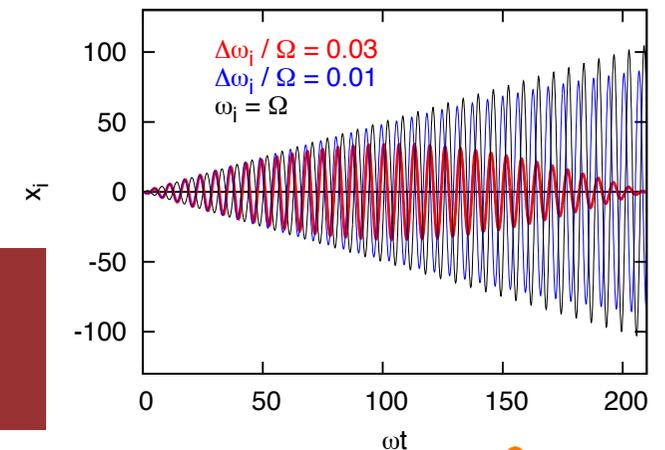
The resonant particles drift away in tune from the resonance as they get excited
