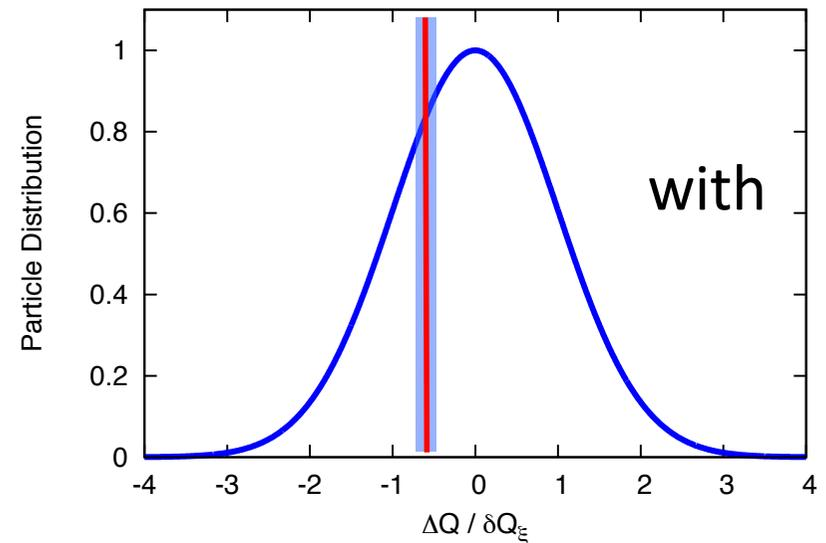
a tune spread does not automatically means Landau Damping
