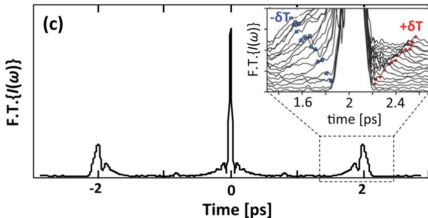
FT of lineout. Inset: Wakefield information is encoded in 2-ps sideband for different densities
