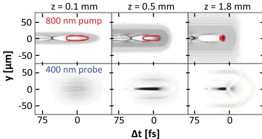
Simulation of wakefield with 800 nm driver evolution (top) and 400 nm FDH probe evolution (bottom)
