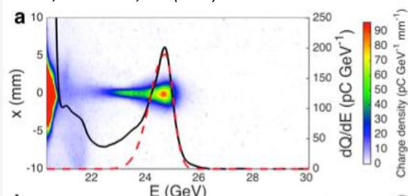
High-density, compressed positron beam for non-linear PWFA experiments. Energy transfer from the front to the back part of the bunch.
