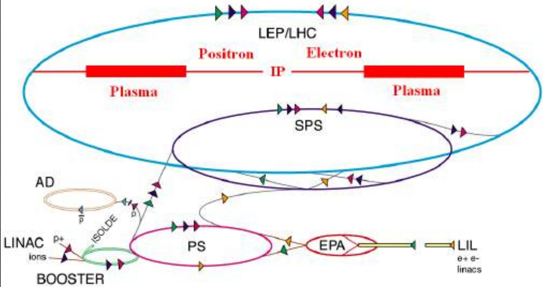
Figure 1: Schematic layout of a 2 TeV CoM electron-positron linear collider based on a modulated proton-driven plasma wakefield acceleration.
