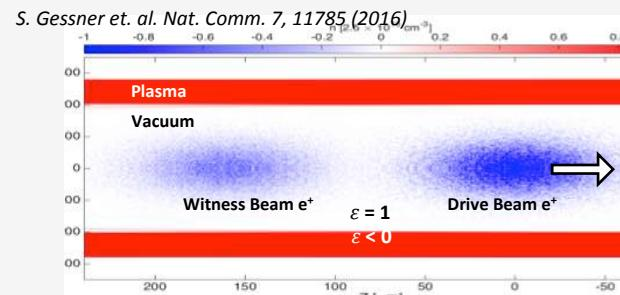
Measurement of **transverse wakefields in a hollow plasma** channel due to off-axis drive bunch propagation.
