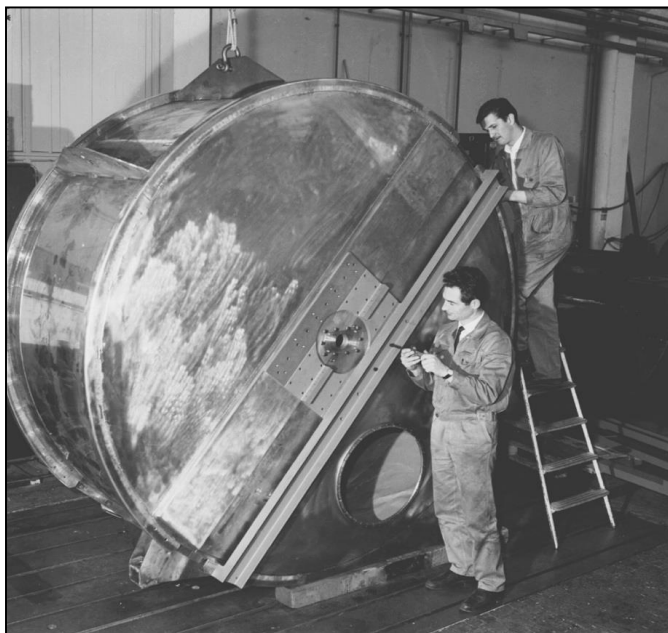
CERN PS 19 MHz Cavity (prototype 1966)
