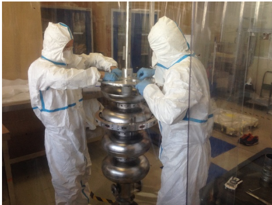
SPL (Superconducting Proton Linac) 704 MHz cavity
