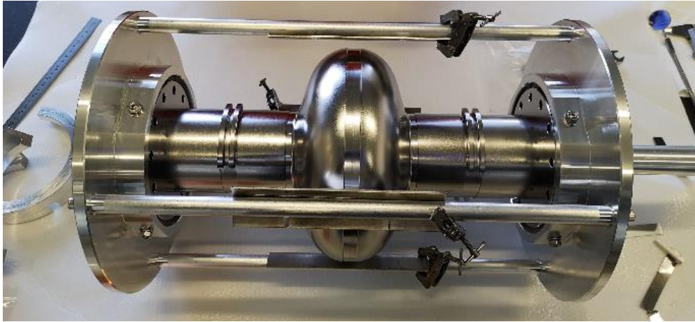
1.3 GHz KEK niobium cavity
