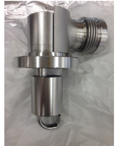
DQW crab cavity and HOM (High-Order-Modes) coupler
