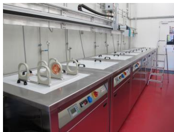
7 sequential cleaning baths with automatized cup handling
