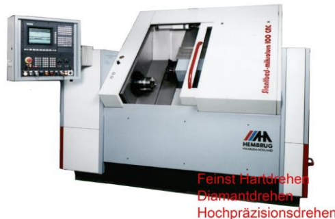
UP-Machine HEMBRUG Slantbed-MIKROTURN-100-CNC Was used to establish the manufacture procedure at PSI Later delivered to the industrial partner for mass production
