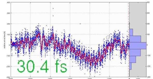
On a short-time scale, the stability is around 30 fs RMS, while on a longer time scale a slow drift is clearly visible and is currently compensated using a feedback based on the BAM.
