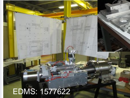
Assemblage and cabling of spare scraper modules
