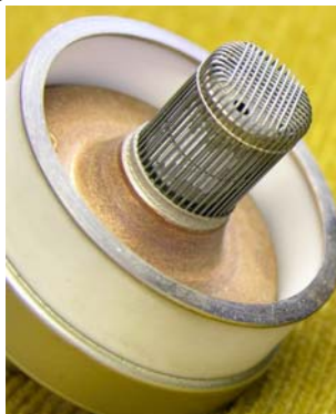
4CX250B (Eimac/CPI), < 500 MHz, 600 W (Anode removed)
