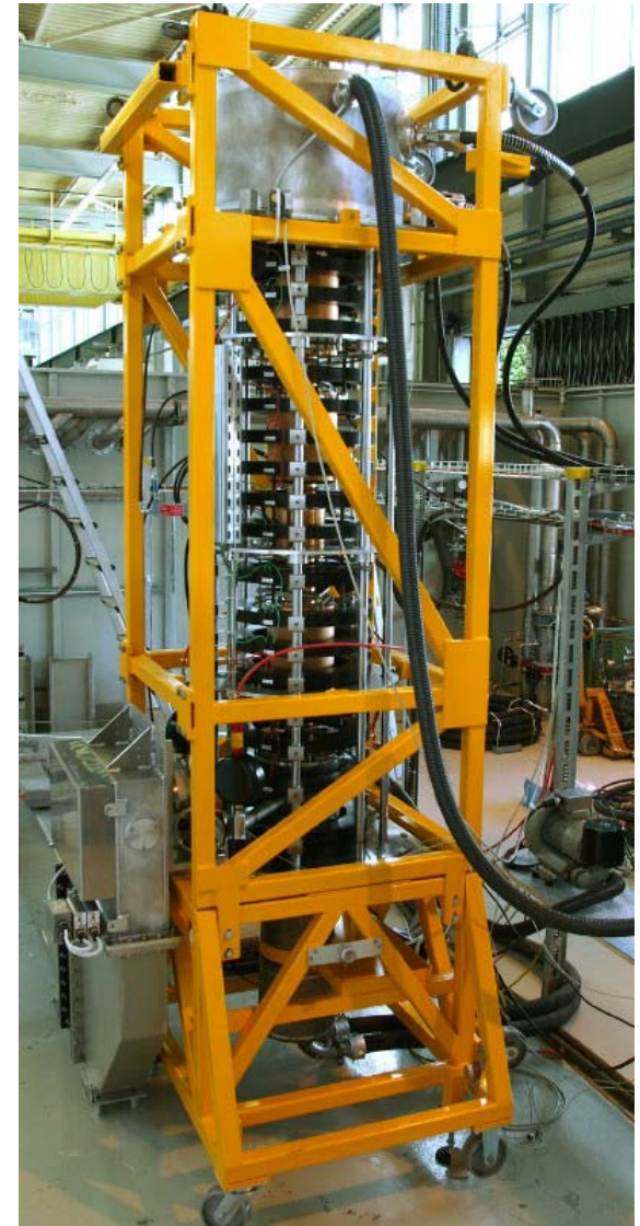
CERN LHC: 400 MHz, 300 kW, CW, \eta 62 %
