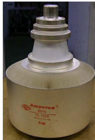
YL1520 (ex Philips, now Richardson), < 260 MHz, 25 kW
