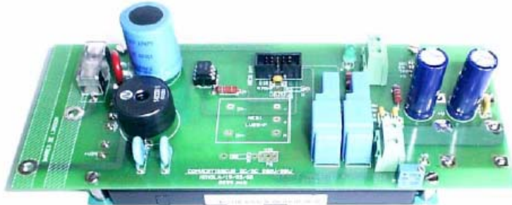
600 W, 300 Vdc / 30 Vdc converter
