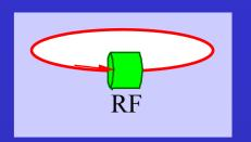
RF cavity provides accelerating field with frequency  $f_{RF} = h \cdot f_0$
