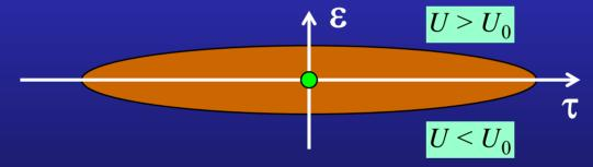
when the particle is in the lower half-plane, it loses less energy per turn, but receives U<sub>0</sub> on the average, so its energy deviation gradually reduces
