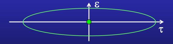
longitudinal coordinate measured from the position of the synchronous electron
