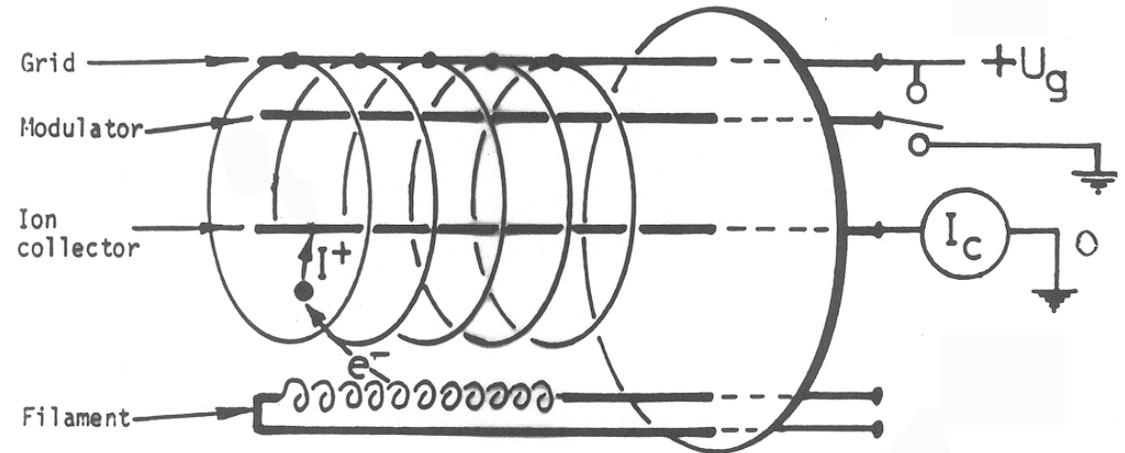
The ionization probability  $P_i$  (number of ion–electron pairs produced  $m^{-1} Pa^{-1}$ ) depends on the type of molecule and on the kinetic energy of the electrons.
