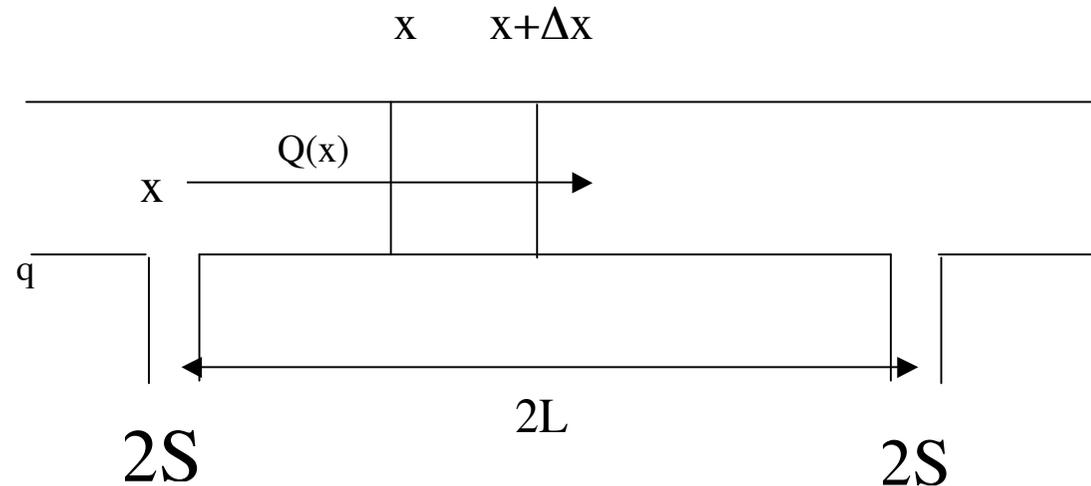
Gas flow:  $Q(x)$  [ $\text{Pa m}^3 \text{s}^{-1}$ ], specific outgassing rate:  $q(x)$  [ $\text{Pa m s}^{-1}$ ]
