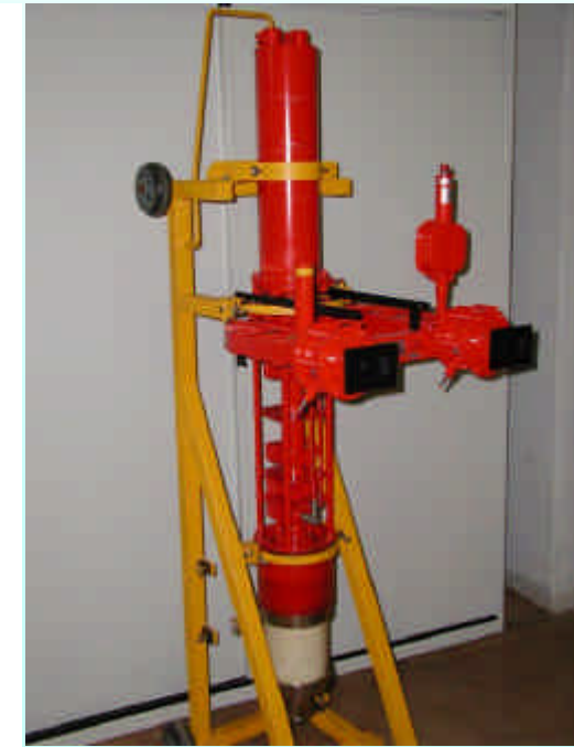
Elettra – Linac Modulator Klystron
