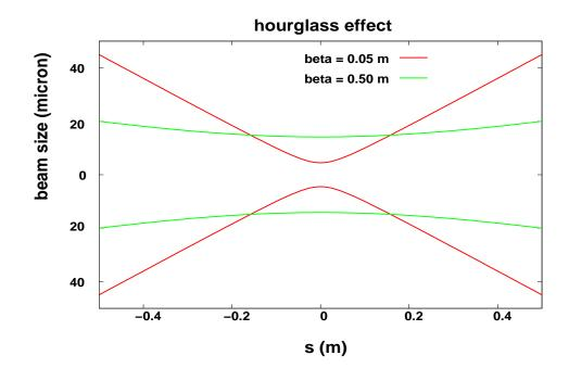
lacksquare Beam size  $\sigma$   $(\propto \sqrt{\beta^*(s)})$  depends on position s
