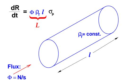
> Interaction rate from flux and target density and size
