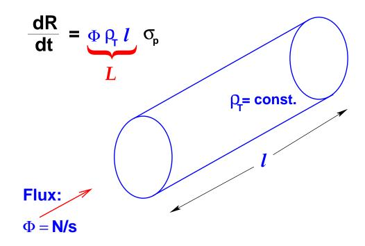
In a collider: target is the other beam ... (and it is moving!)
