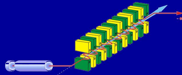
**A Free Electron Laser is a device that converts a fraction of the electron kinetic energy into coherent radiation via a collective instability in a long undulator**
