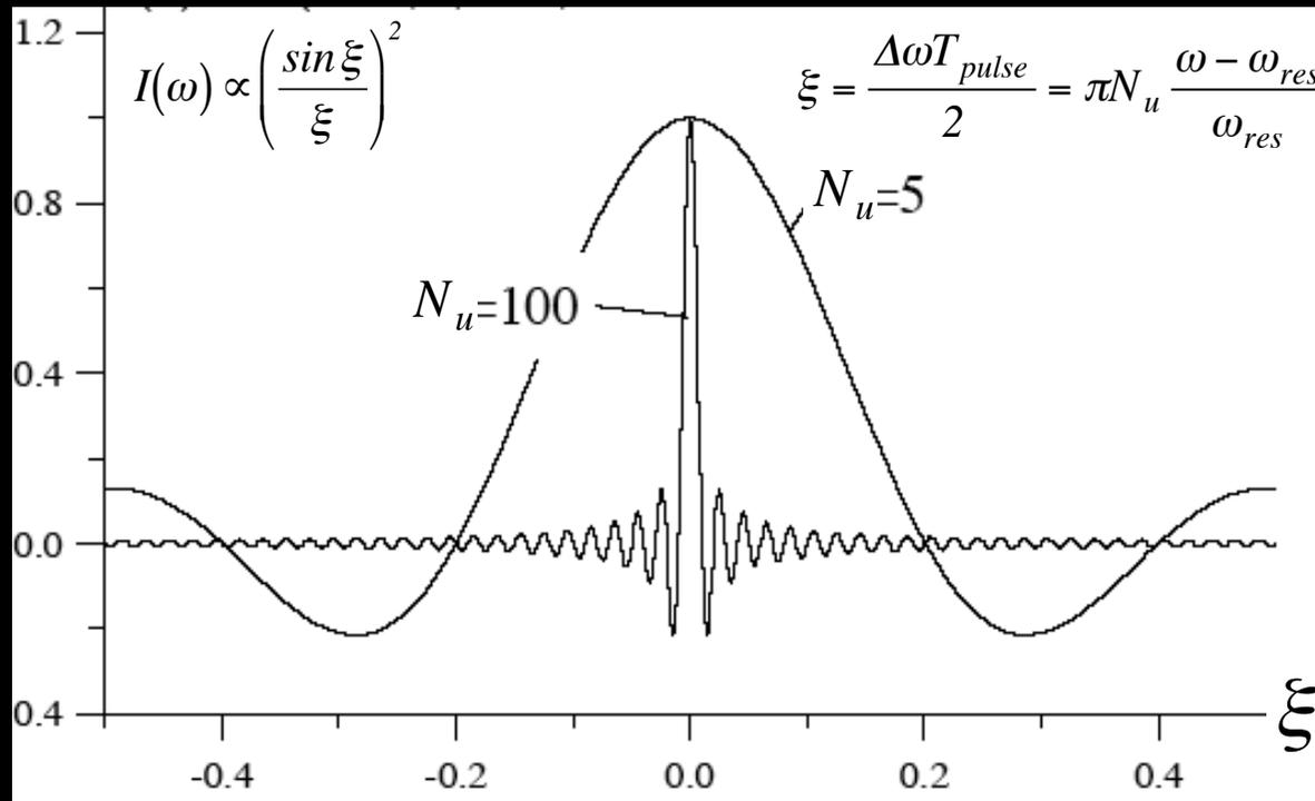
$$\frac{\Delta\omega}{\omega} \approx \frac{1}{N_u} \quad \text{Line width}$$
