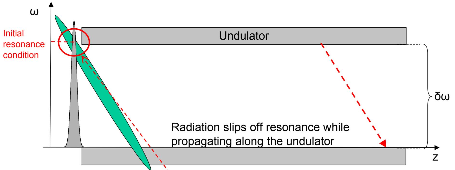
Resonance condition is a function of Beam energy (chirp) / Undulator K (untapered)
