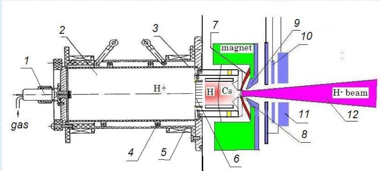
1- *gas valve*; 2- *discharge volume*; 3- *discharge vessel*; 4- *helicon saddle like antenna*; 5- *magnetic coil*; 6- *ion/atom converter*; 7- *electron flux*; 8- *emission aperture (slit)*; 9- *extraction electrode*; 10-*suppression /steering electrode*; 11- *ion beam*.
