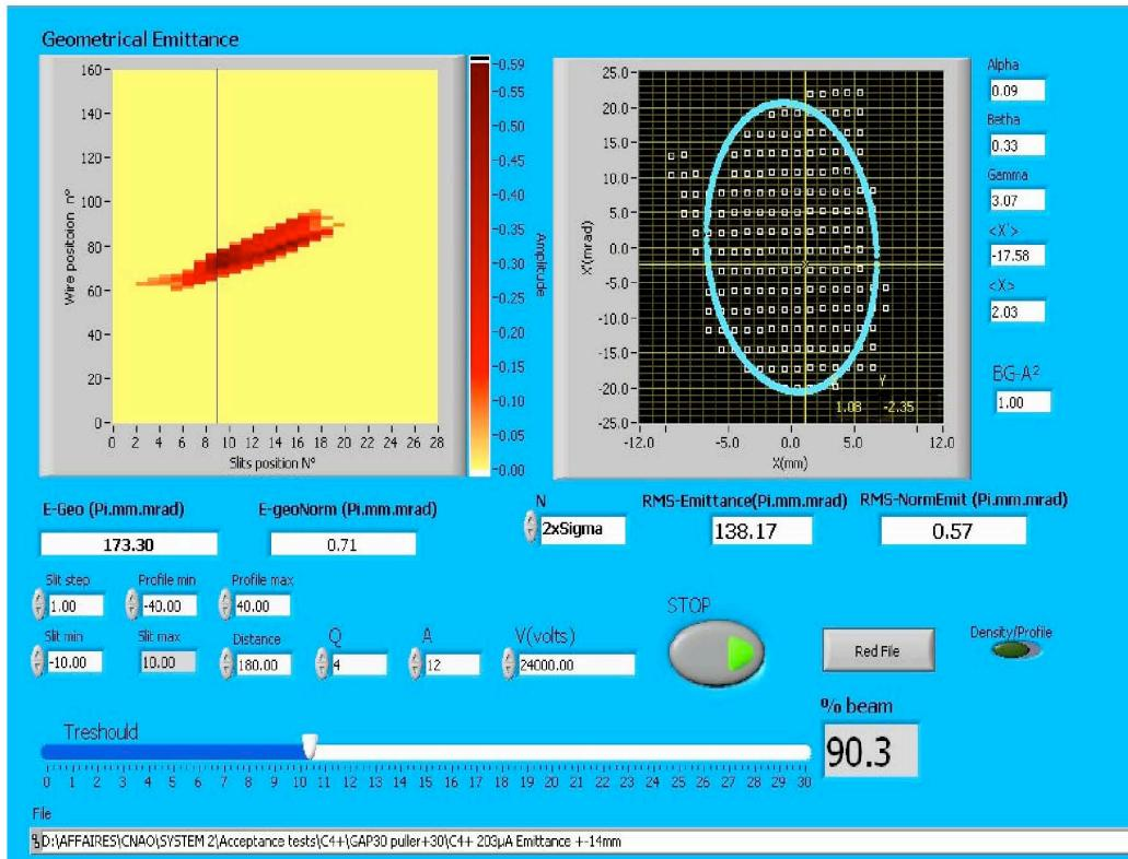
Figure 36:  $12C^{4+}$  Emittance with the new gap.
