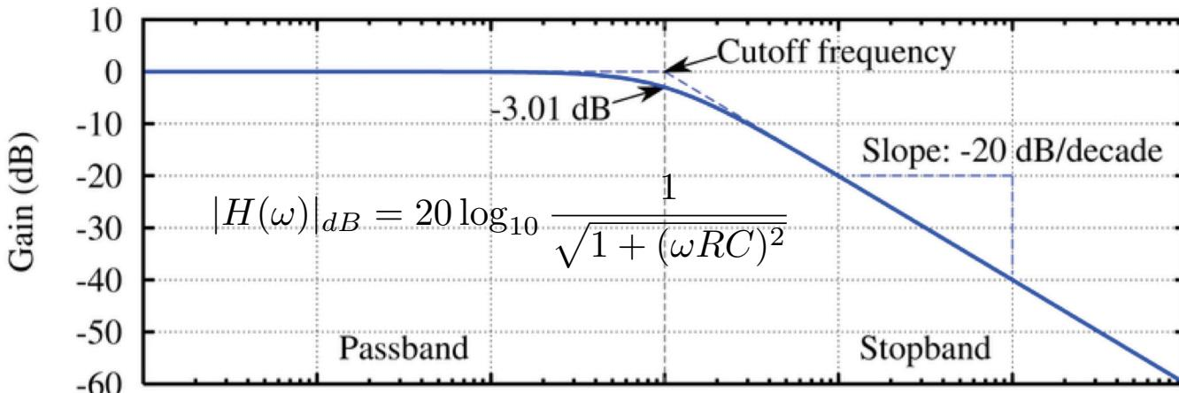
$$\frac{V_{out}}{V_{in}} = \frac{1}{1 + j\omega RC}$$
