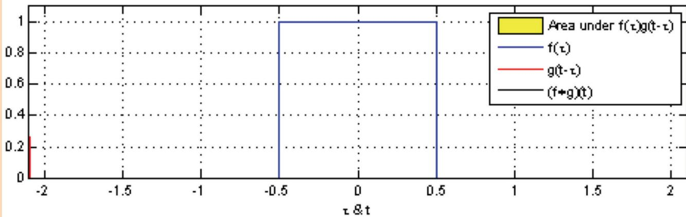
In this depiction,  $f(\tau)$  could represent the response of an RC circuit to a narrow pulse that occurs at  $\tau = 0$ . In other words, if  $g(\tau) = \delta(\tau)$ , the result of convolution is just  $f(t)$ . But when  $g(\tau)$  is the wider pulse (in red), the response is a "smeared" version of  $f(t)$ . It begins at  $t = -0.5$ , because we defined  $t$  as the distance from the  $\tau = 0$  axis to the center of the wide pulse (instead of the leading edge).
