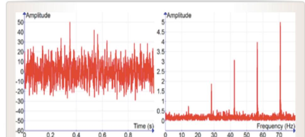
The signal on the left looks like noise, but the signal processing technique known as the [Fourier transform](#) (right) shows that it contains five well defined frequency components.
