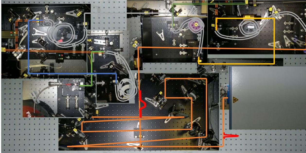
Vertical breadboard at beam pipe
