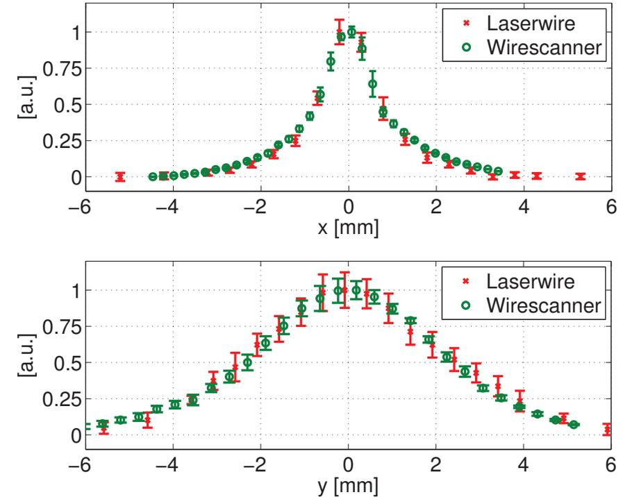
Figure 6: Beam profiles recorded with the laserwire and a wire-scanner in both planes. As the wire scanner is located 2.7 m downstream of the laserwire, its profile is scaled according to the beta-function ratio of both locations.
