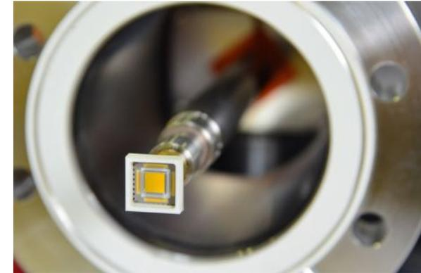
Figure 8: sCVD diamond detector [12] mounted on the actuator that is part of the laser monitor assembly for the 50 MeV experiment.
