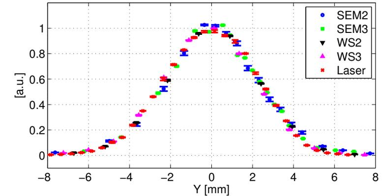
Figure 11: Overlay of 107 MeV H<sup>-</sup> beam  $\sigma$ -scaled profiles recorded with different devices.
