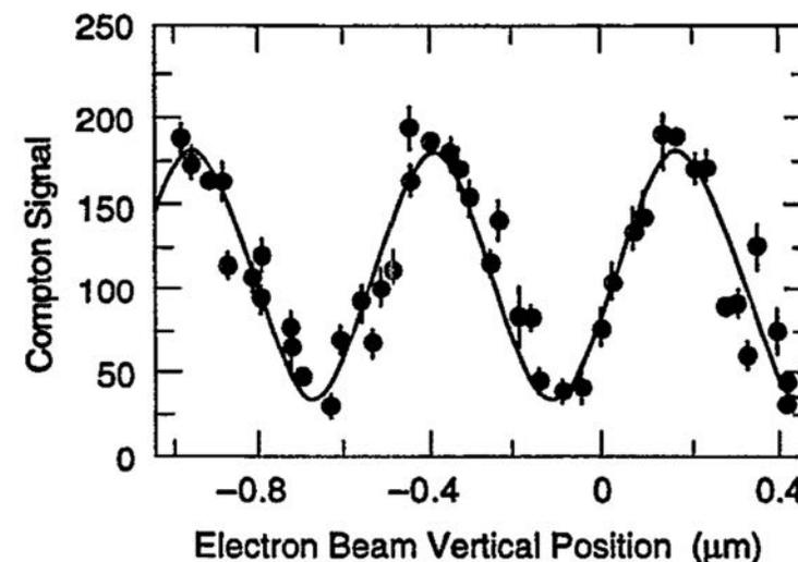
FIG. 2. Measurement of the vertical height of the beam at the FFTB focal point with the laser-Compton spot monitor. The observed fringe spacing agrees well with the 0.5  $\mu\text{m}$  expected from the wavelength of the laser. The beam height is determined from the ratio of the Compton signal at the minima of the fringe pattern to the signal at the peaks of the pattern. In this case, the beam height is 73 nm.
