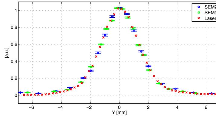
Figure 10: Comparison of SEM-grid  $\sigma$ -scaled profiles with the laserwire profile for the 80 MeV H<sup>-</sup> beam.
