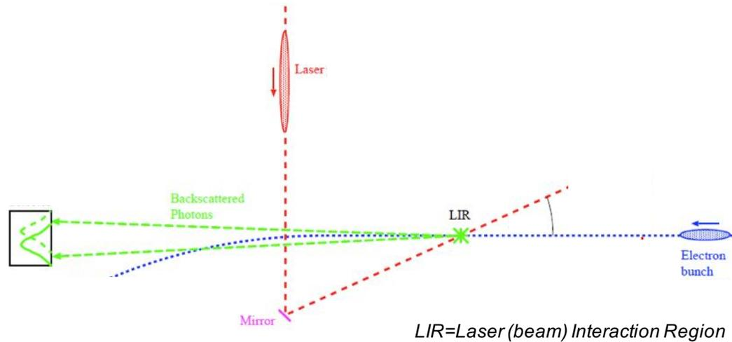
$\gamma$  profile and asymmetry (R/L laser helicity) at LEP
