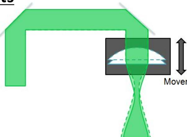
focal scan in y : Res. 0.1μm
