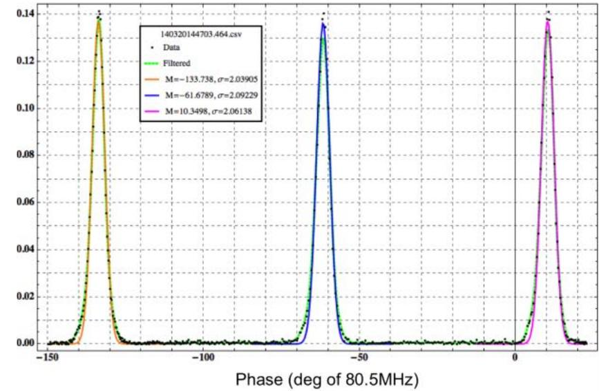
Figure 3: Typical bunch profile taken with phase shift technique. Peaks are distributed 72° apart.
