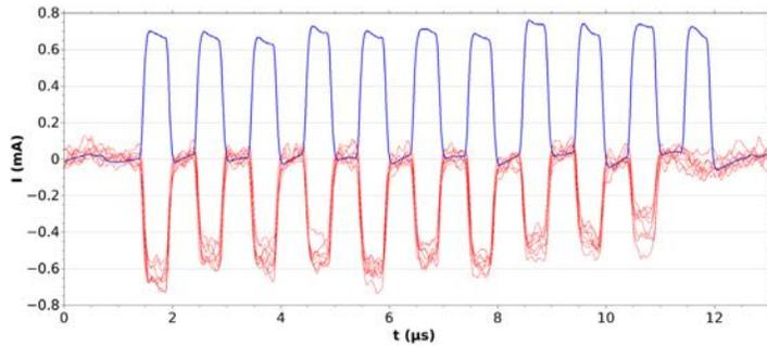
FIG. 4. The experimental results. The average beam current for a 11  $\mu\text{s}$  H<sup>-</sup> beam measured by the beam current monitor at the interaction point before stripping (blue), and eight separately measured stripped proton beam pulses on the same beam current monitor during stripping (red).
