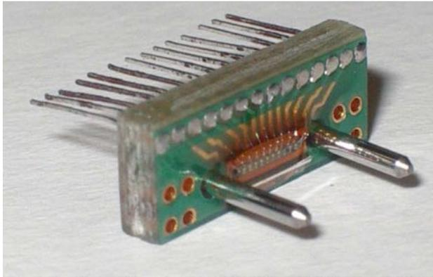
Fig. 3. Photograph of a VCSEL array mounted on a base PCB with the MT guide pins.
