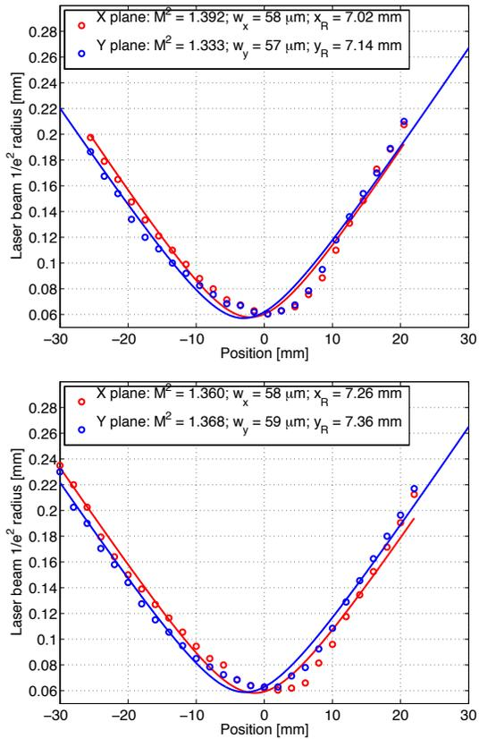
Fibre lengths set to illuminate IP in X & Y at slightly different times:
