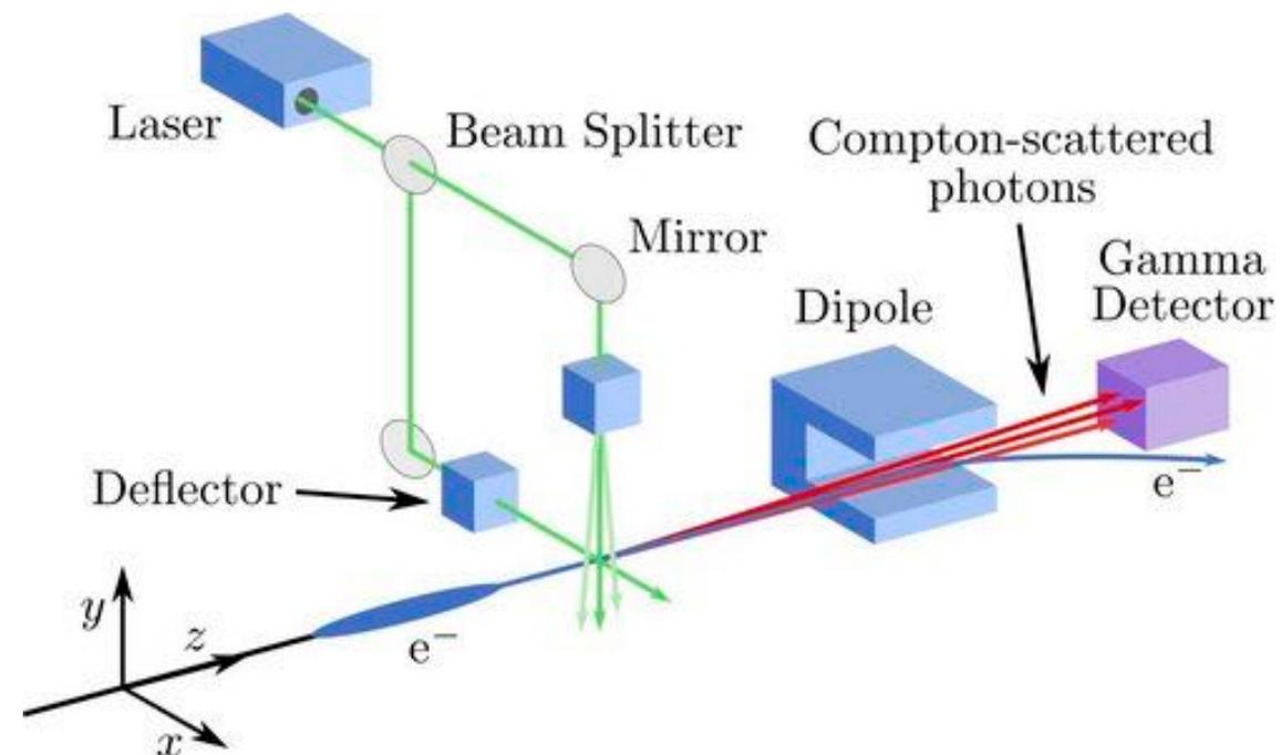
*Laser beam must be focused to a size compatible with the particle beam profile*
