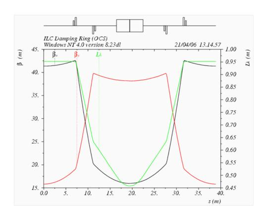
Outside the dipole, the dispersion is relatively large. This is not ideal for a light source, since insertion devices at locations with large dispersion will blow up the emittance.
