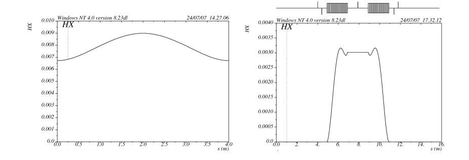
The curly-H function is much smaller in the DBA lattice (right) than in the FODO lattice (left).
