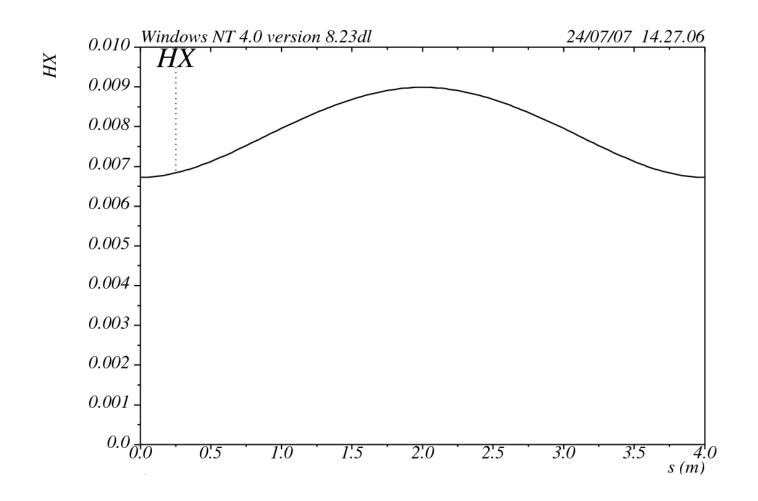
As a first attempt at reducing the natural emittance, we can try reducing the curly-H function in the dipoles, by designing a lattice that has zero dispersion at either end of a dipole pair.
