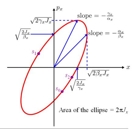
Applying simple geometry to the phase space ellipse, we find that the action (for uncoupled motion) is related to the Cartesian variables for the particle by:
