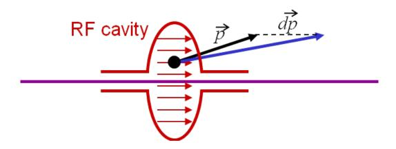
Fortunately, RF cavities are usually designed to provide a longitudinal electric field.
