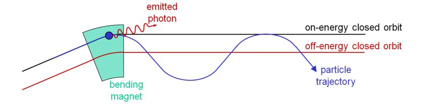
The beam eventually reaches an equilibrium distribution determined by a balance between the radiation damping and the quantum excitation.
