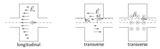
In our cavity mode Ix induces  $E_z$  giving a longitudinal impedance  $Z_L$ . Excitation at distance  $x_0$  gives a gradient of the  $\partial E_z/\partial x$  related to  $Ix_0$  by a factor k
