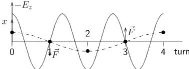
B) A cavity is tuned to lower sideband. The bunch traverses it next turn in situation 'B',  $t=T_r(k'+3/4)=T_r(k'+1-1/4)$  with negative velocity and a force in same direction. This increases its velocity and leads to instability.
