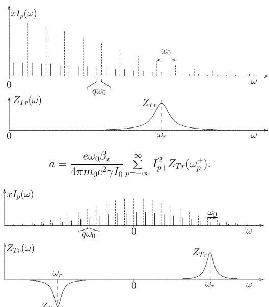
To drive this instability we need a narrow band impedance with a memory lasting at least for one turn.
