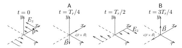
A bunch p traverses a cavity with off-set x, excites a field  $\vec{E}$  which converts after  $T_r/4$  into a field  $-\vec{B}$ , then into  $-\vec{E}$  and after into  $\vec{B}$ . The bunch oscillates with tune Q having a fractional part q=1/4 seen as sidebands at  $\omega_0(\mathrm{integer}\pm q)$  by a stationary observer.
