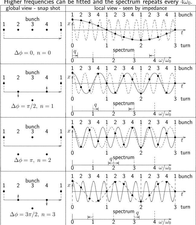
The side-band frequencies of M bunches oscillating in a mode n, obtained by a graphical method, are
