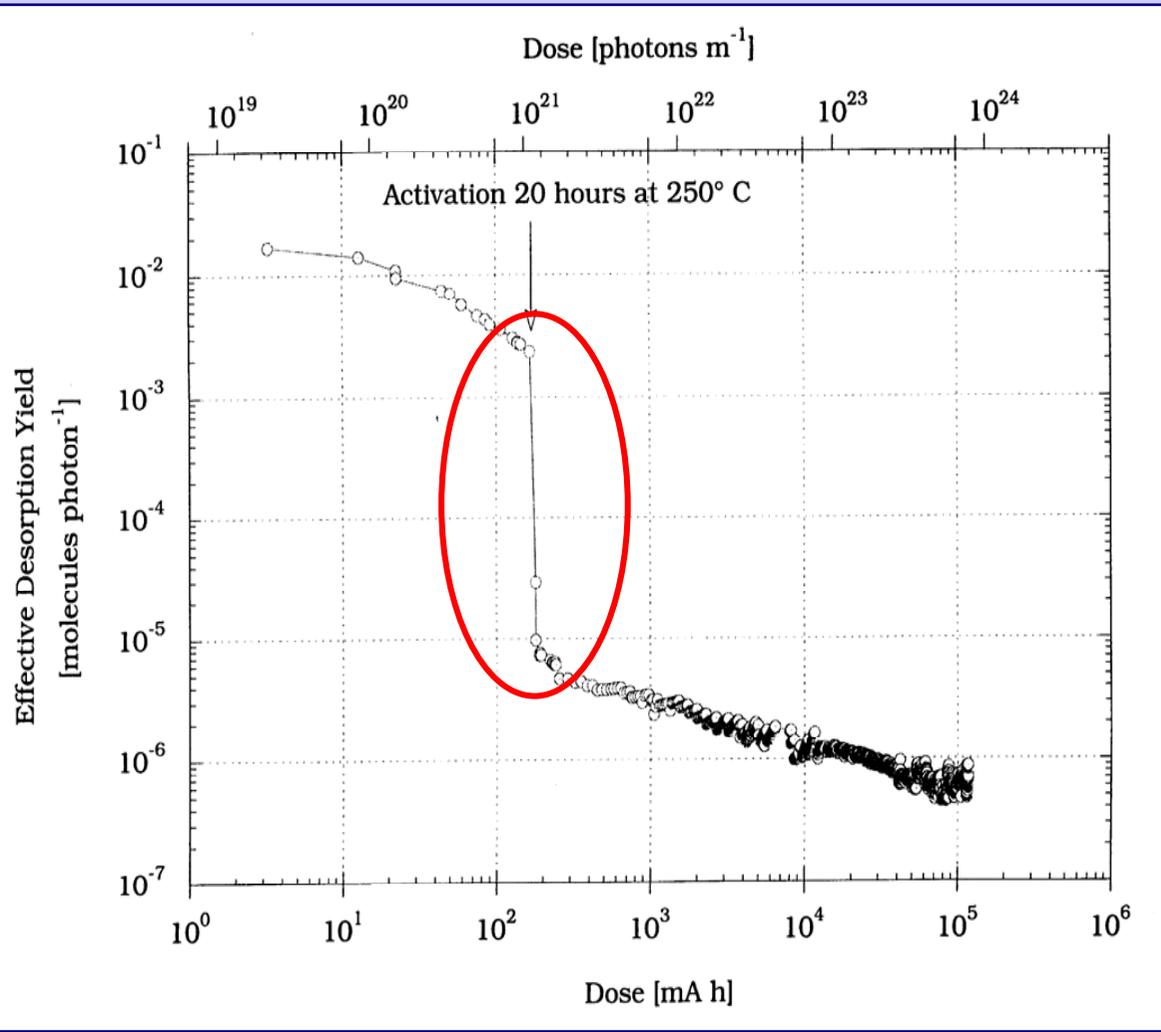
“Variation of the effective molecular desorption yield as a function of the beam and photon dose measured on a TiZrV coated stainless steel chamber installed on a beamline at ESRF Grenoble.
