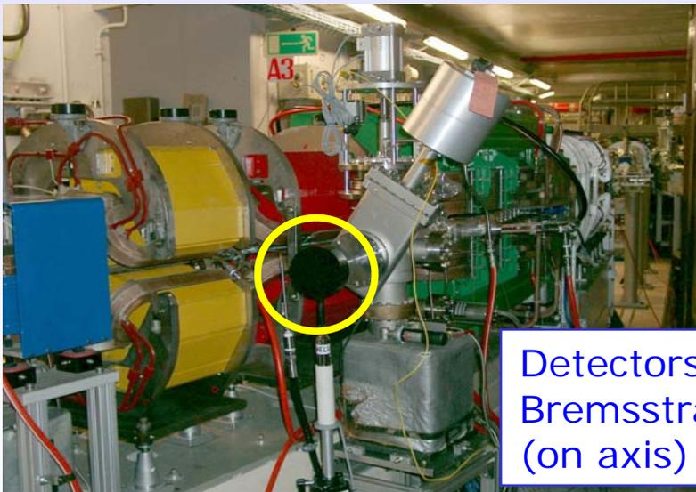
Detectors for Bremsstrahlung (on axis)
