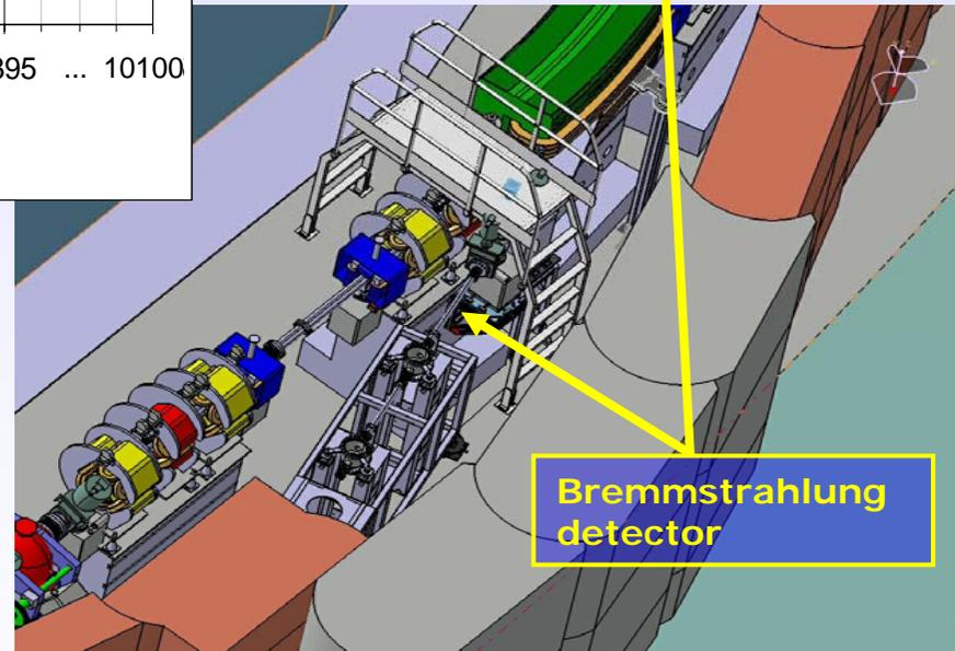
In a particle accelerator, the measurement of the gas-bremsstrahlung provides an indirect information about the total pressure inside the vacuum chamber.
