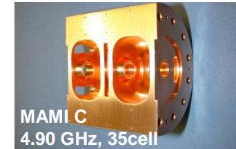
**cw high current operation hampered by limited HOM damping capabilities**
