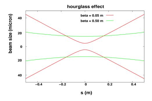
Beam size  $\sigma \quad (\propto \sqrt{\beta^*(s)})$  depends on position s
