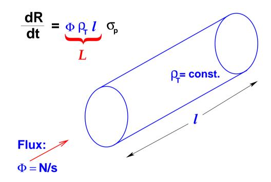
Interaction rate from <u>flux</u> and <u>target density</u> and <u>size</u>
