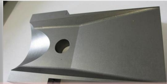
Collimator upgrade for LHC → reduction of the transverse impedance contribution of the collimator jaws → new proposed material MoGr.
