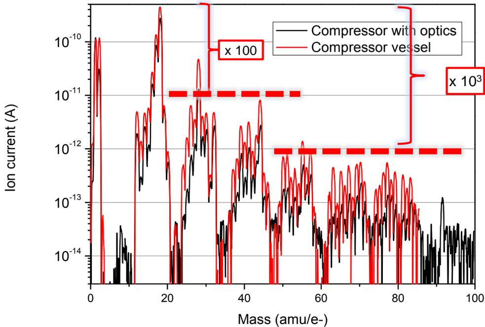
Residual Gas Analysis: after few hours of filament conditioning, the amplitude of the peaks is compared to the water content in the system. The component is considered accepted if the ratio between the water peak and the peaks up to mass 44 is higher than 100 and if the same ratio is higher then 1000 for peaks above mass 44.
