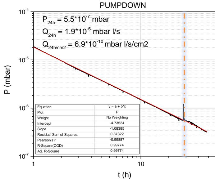
Pump down curve: outgassing rate value at 24h in N<sub>2</sub> equivalent to be compared with the acceptance criteria for each specific accelerator and transfer line.
