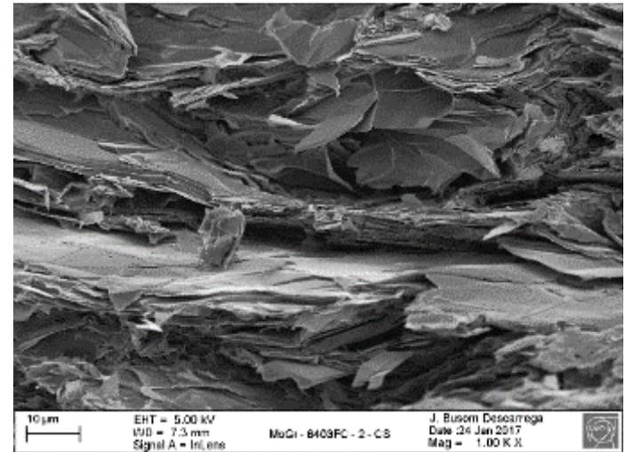
Focus Ion Beam and SEM analysis to evaluate the presence of voids, pores and surface damages induced by machining.
