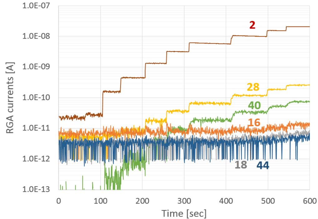
In case of long coated beam pipe need to carefully consider the cleanliness of the injection line and presence of hot filaments or selective pumping in the system.
