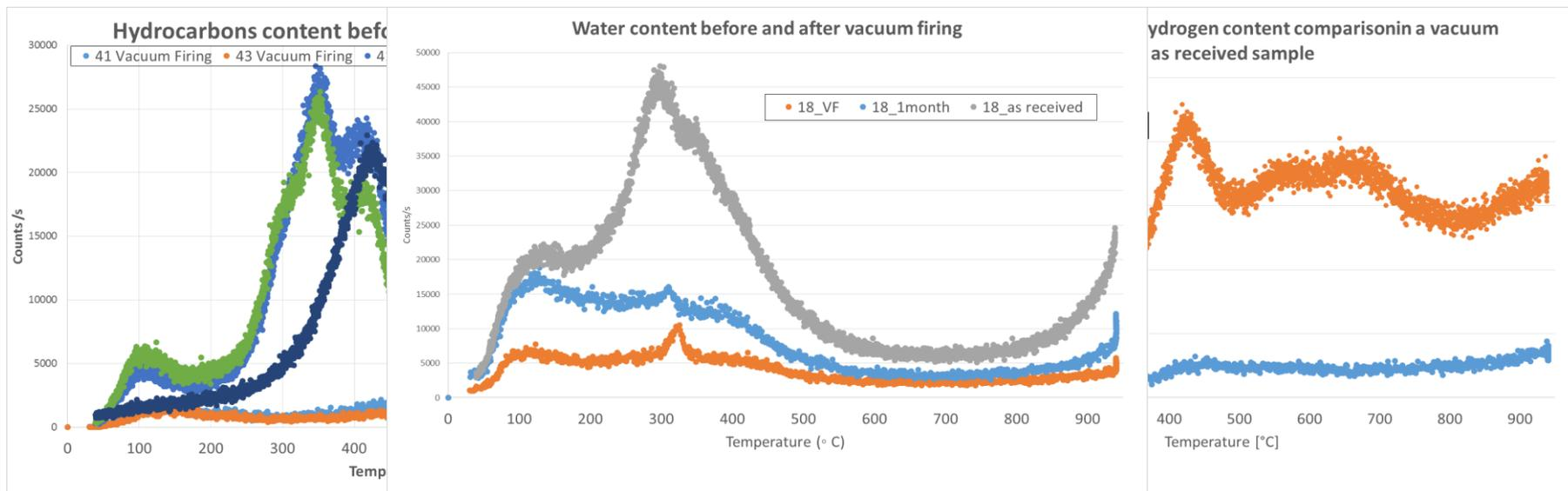
TDS (Thermal desorption spectroscopy) is used to study gases evolution from the material under different conditions (before and after vacuum firing, air time exposure..).
