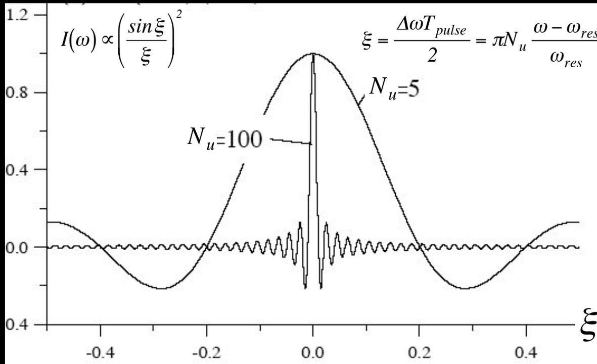
$$\frac{\Delta\omega}{\omega} \approx \frac{1}{N_u} \quad \text{Line width}$$
