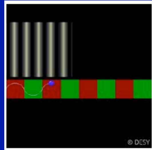
After one wiggler period the electron sees the radiation with the same phase if the flight time delay is exactly one radiation period:  $\Delta t = t_e - t_{ph} = T_{rad}$
