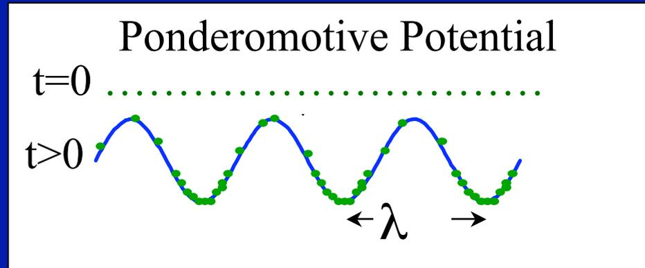
The phase of the combined "ponderomotive" (radiation + undulator) field, propagates in forward direction with a phase velocity that corresponds to the velocity of the resonant particle:
