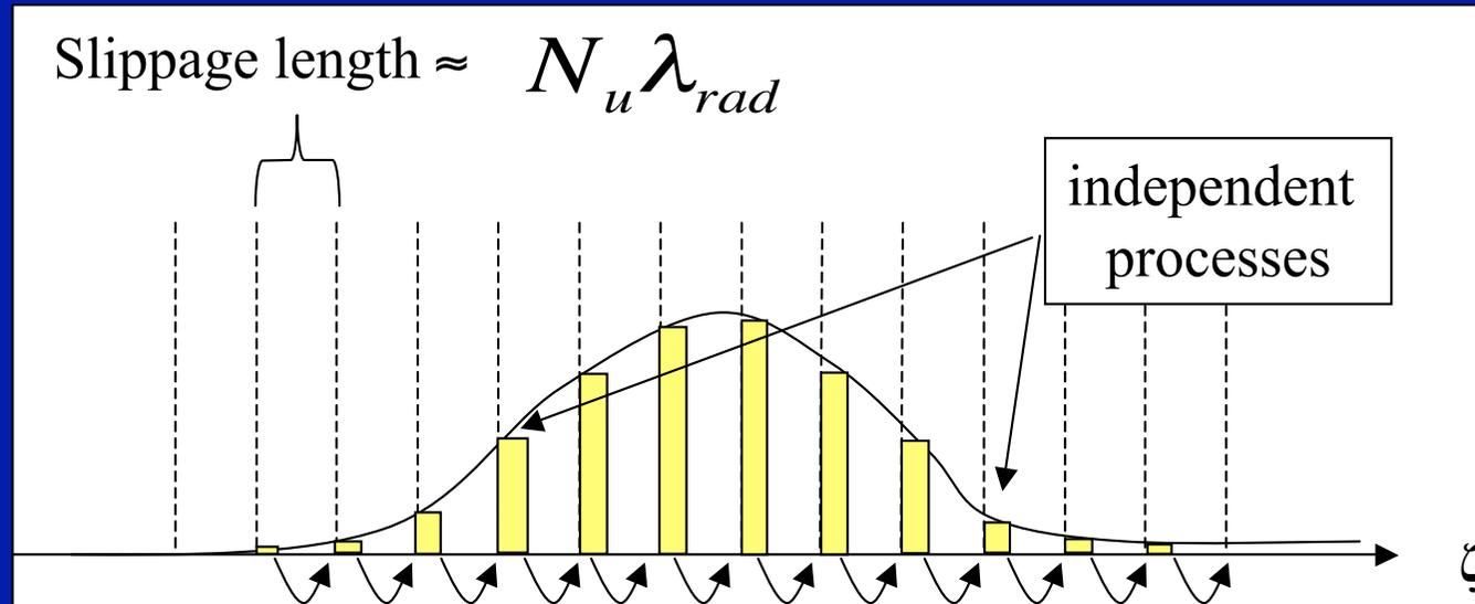
The radiation "slips" over the electrons for a distance  $N_u \lambda_{rad}$
