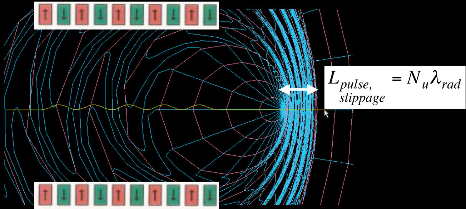
Due to the finite duration the radiation is not monochromatic but contains a frequency spectrum which is obtained by Fourier transformation of a truncated plane wave
