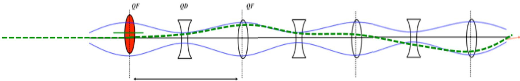
**In a Linac or Transfer Line** – starting with a perfect orbit – the misaligned quadrupole creates an oscillation that is transformed from now on downstream via
