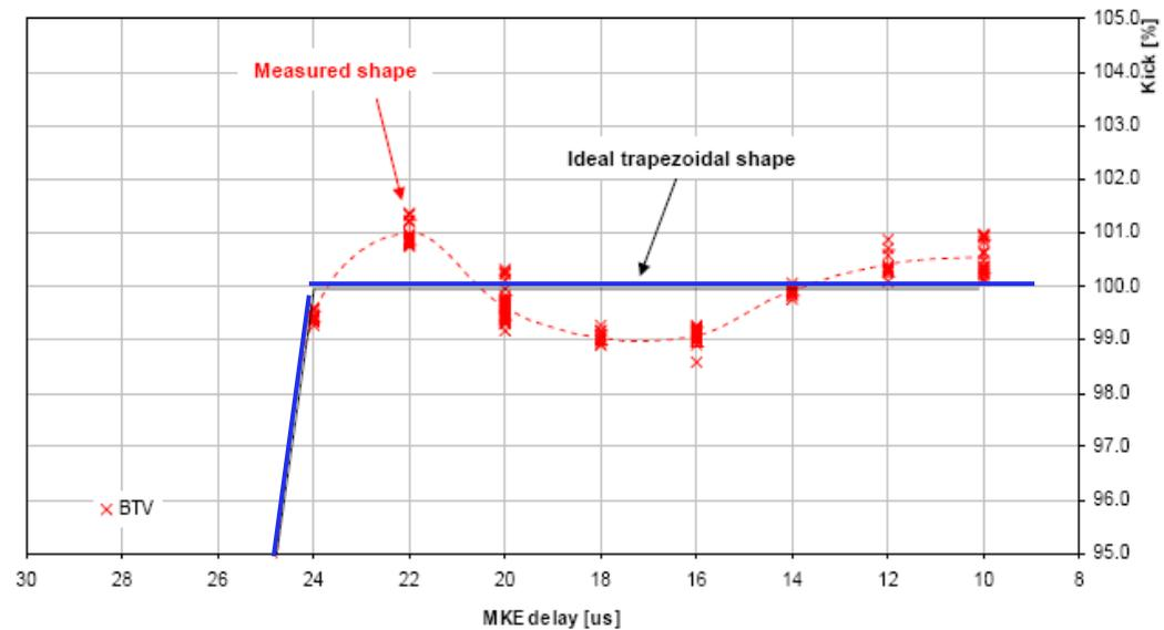
**Kicker "plateau" at the end of the PS - SPS transferline measured via injection - oscillations**
