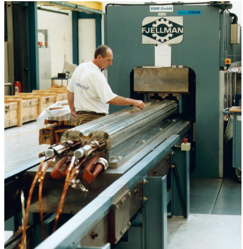
LHC dipole collaring
