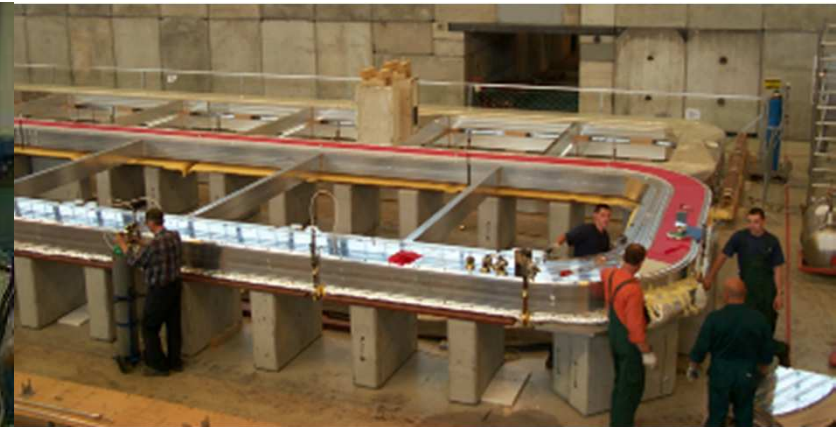
BT coil encasing at CERN
