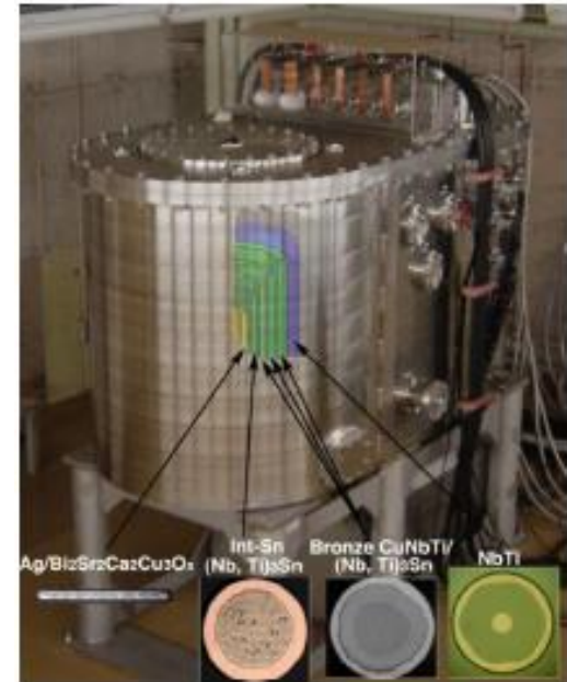
Cryogenfree 18 T superconducting magnet with a Bi2223 insert
