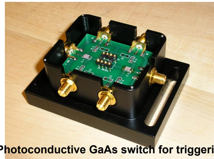
Photoconductive GaAs switch for triggering
