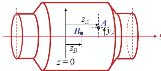
The transverse forces in a particular component are described by a transverse wake function  $W_{\perp}(z)$ , defined so that:
