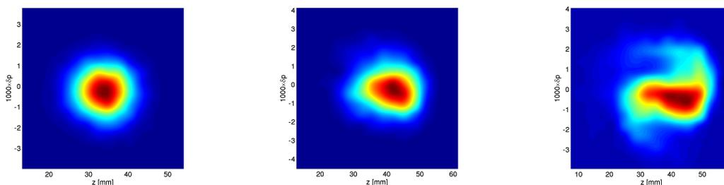
Tracking simulation of longitudinal phase space distribution in a storage ring with wake fields, and (left to right) increasing bunch population.
