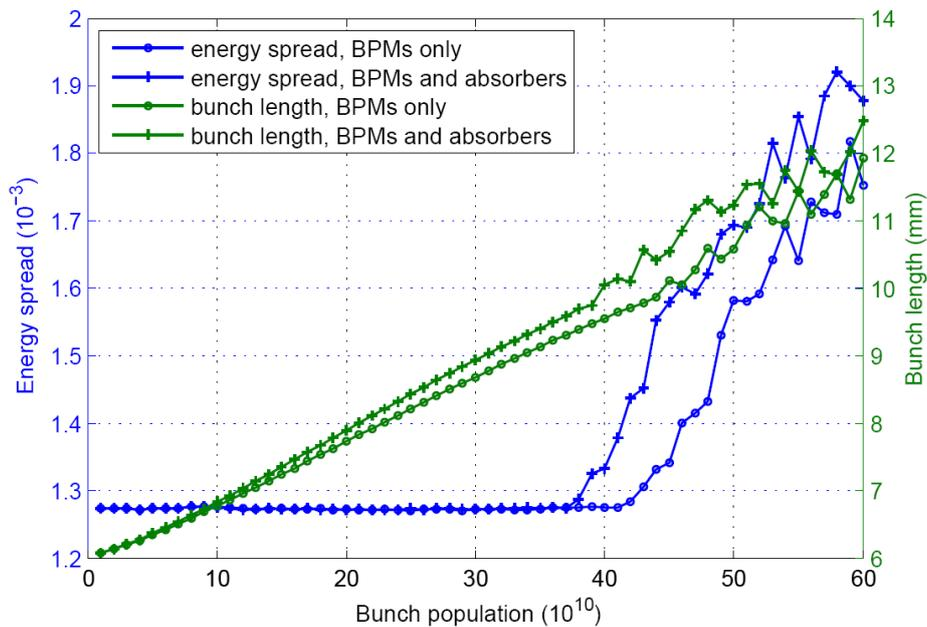
Energy spread and bunch length as functions of bunch population in the ILC damping rings, with two different impedance models.
