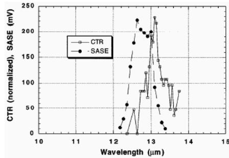
FIG. 3. SASE and CTR signals as a function of wavelength, with CTR scaled to SASE amplitude.
