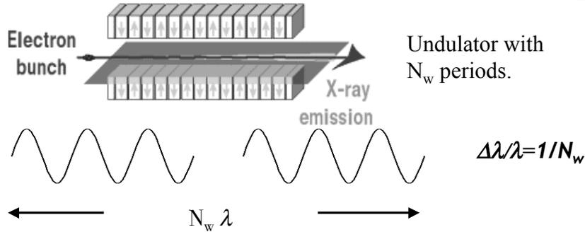
Each electron emits a wave train with  $N_w$  waves
