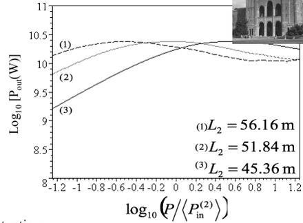
Shot-to-shot fluctuations of output radiation power are reduced by operating the FEL amplifier in the non-linear regime.
