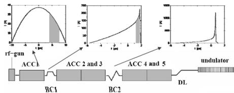
Strong energy chirp along current spike leads to significant shortening of the radiation pulse. Minimum pulse length occurs in the end of the linear regime.
