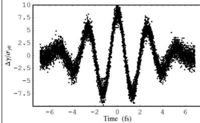
Modulating Laser at wavelength 2.2 mm, power 6 GW
