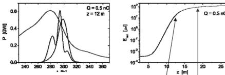
The VUV FEL is capable to produce short, down to 20 fs radiation pulses with GW-level peak power and degree of contrast 80 %:
