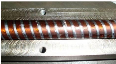
Nb3Sn short prototypes will be constructed soon (1.5T @ 11.5mm?)
