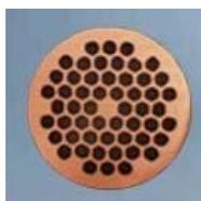
NbTi/Cu wire cross section
