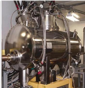
Photo of SC wiggler installed on CLS storage ring.
