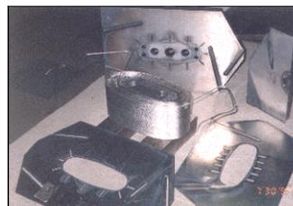
Nb<sub>3</sub>Sn/Cu coil after baking out
