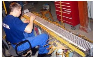
Magnet array of horizontal racetrack type poles (example of 30 mm period SC 2.1T wiggler)
