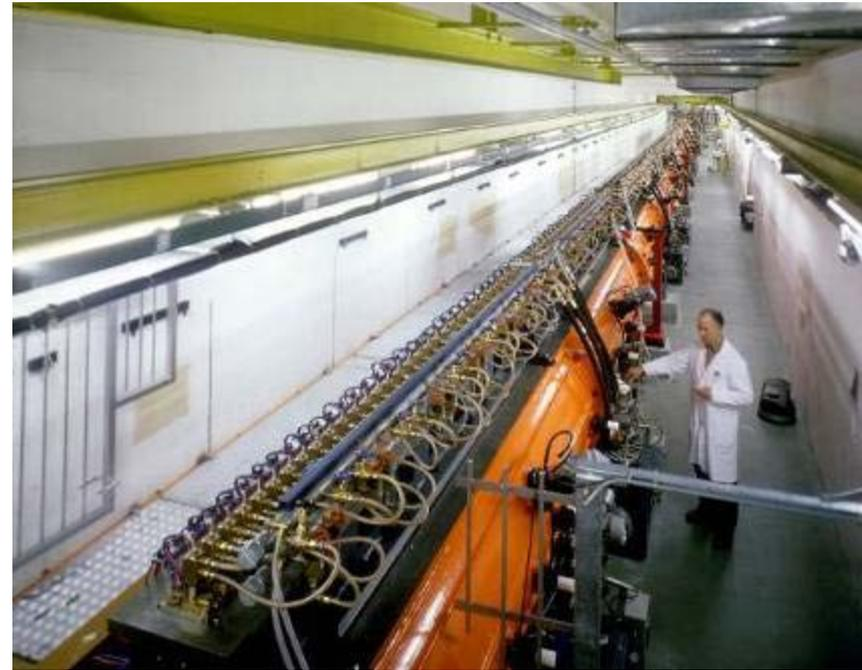
**Top; CERN Linac2 Drift Tube Linac accelerating tank 1 (200 MHz). The tank is 7m long (diameter 1m) and provides an energy gain of 10 MeV.**
