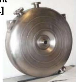
Superconducting linacs for low and medium beta ions are made of multi-gap (1 to 4) individual cavities, spaced by focusing elements. Advantages: can be individually phased → linac can accept different ions
