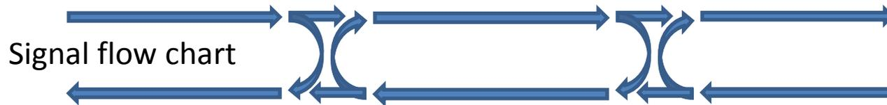
Reflections from notches lead to a superimposed standing wave pattern.
