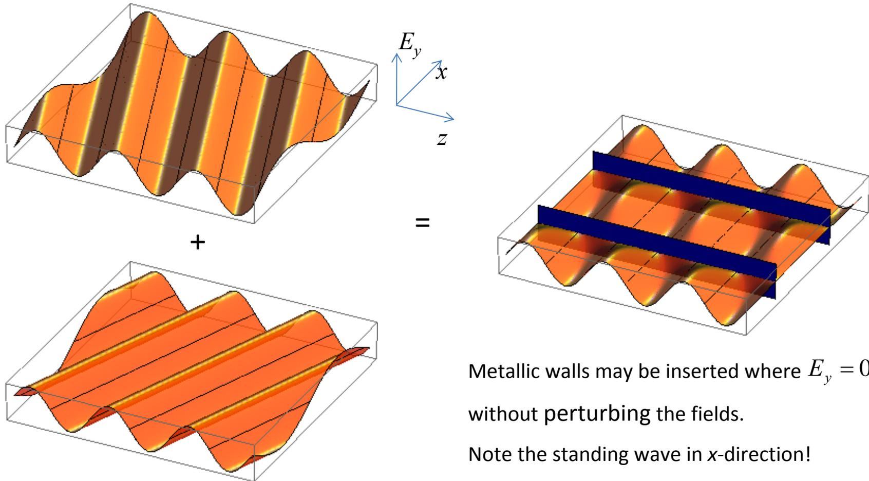
Metallic walls may be inserted where  $E_y = 0$  without perturbing the fields.
