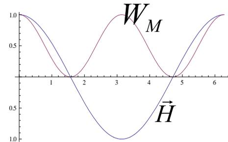
Since  $\vec{E}$  and  $\vec{H}$  are 90° out of phase, the stored energy continuously swaps from electric energy to magnetic energy. On average, electric and magnetic energy must be equal.
