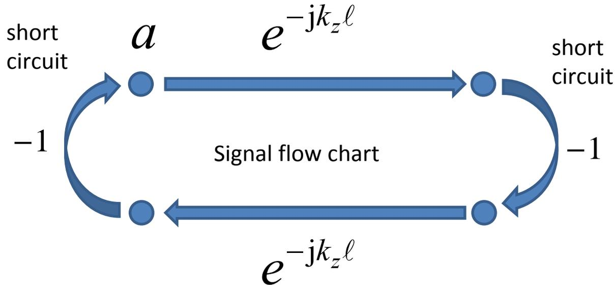
Eigenvalue equation for field amplitude  $a$ :
