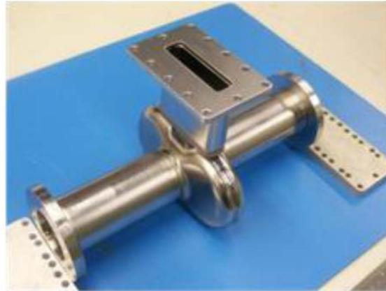
On-cell damping involves coupling directly into the cavity cell as opposed to the beam-pipe as is common in most elliptical cavities.
