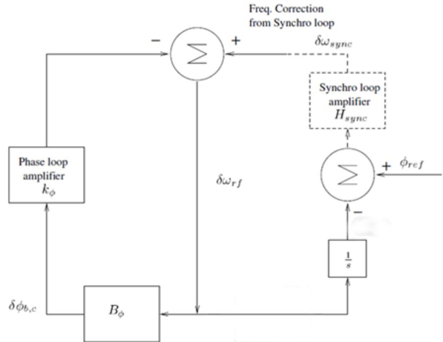
Block diagram of the Phase-Synchro loop in Laplace transforms
