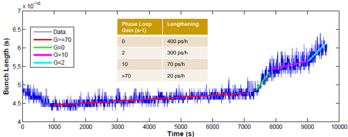
LHC single bunch at 3.5 TeV  $1E10$  p. Evolution of bunch length with time as a function of the Phase Loop gain. Fixed 8 MV RF (T. Mastorides, P. Baudrenghien, May 2010). LHC BQM system.
