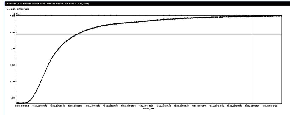
The 45 min long LHC frequency ramp from 450 GeV (400.788860 MHz) to 3.5 TeV (400.789 713 MHz)
