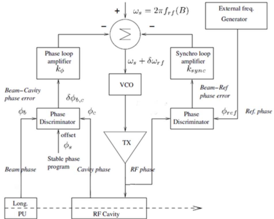
Another classic combination for proton and ion synchrotrons: Phase loop and Synchro loop
