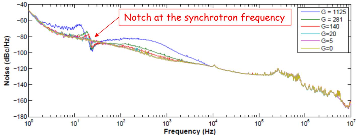
PSD of the phase noise in dBc/Hz in a LHC cavity with circulating 3.5 TeV bunch, for various phase loop gains (in  $s^{-1}$ ), 1.66 MV. The synchrotron frequency is  $\sim 24$  Hz
