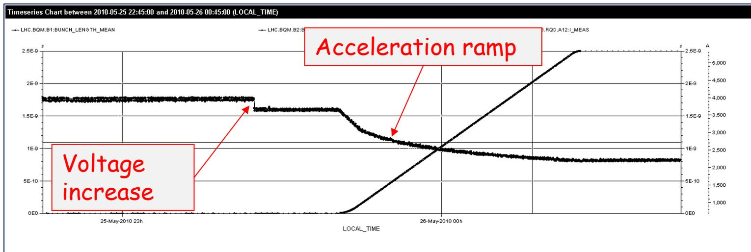
Bunch length evolution in the LHC: capture at 450 GeV with 3.5 MV, voltage increase to 5 MV before start ramp then rise to 8 MV in first part of the ramp (up to 3.5 TeV). Bunch length ( $4\sigma$ ) B1: 1.82 ns  $\rightarrow$  1.61 ns  $\rightarrow$  0.83 ns / B2: 1.75 ns  $\rightarrow$  1.58 ns  $\rightarrow$  0.77 ns Measured by the LHC Beam Quality Measurement (BQM) system, G. Papotti
