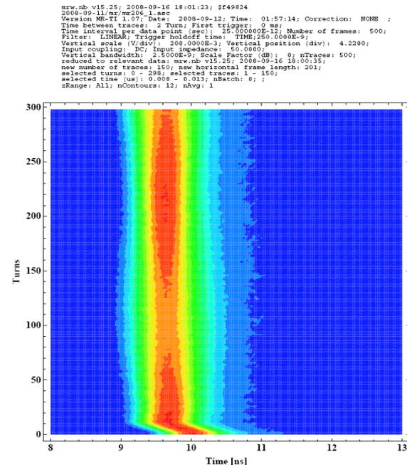
Sept 12, 2008. First capture of LHC ring 2 beam with Phase Loop ON. Left: Phase error. Right: Mountain range display. Notice the rapid damping of the injection phase error and the lasting quadrupole oscillations caused by voltage mismatch (see next slides). Courtesy of T. Bohl
