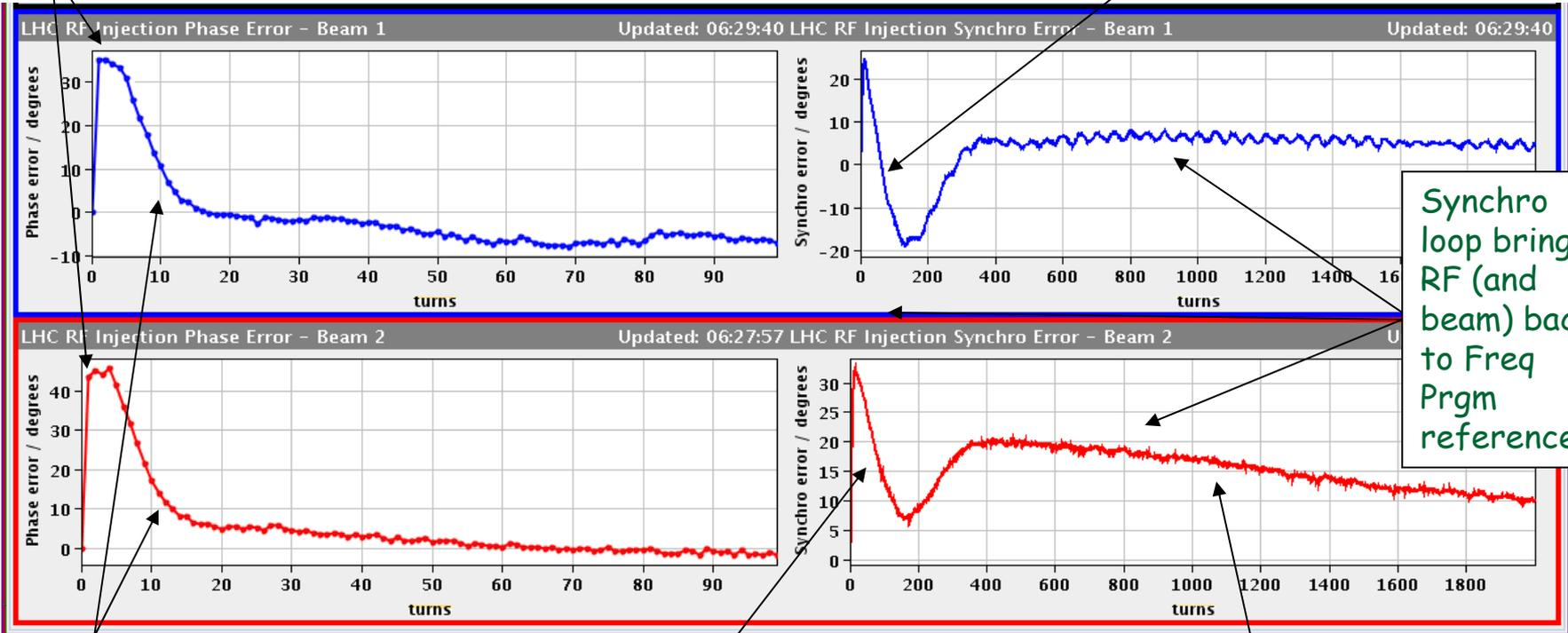
Synchro loop brings RF (and beam) back to Freq Prgm reference
