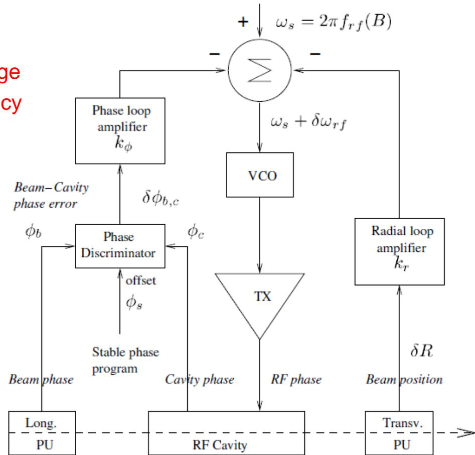
A classic combination for proton and ion synchrotrons: Phase loop and Radial loop
