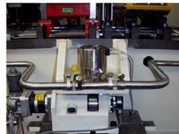
Figure 4: HLS sensor with water pipe connection.
