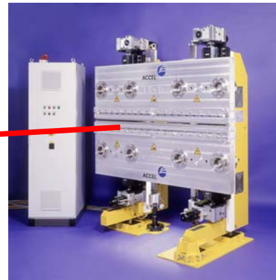
undulator: radiation source (PETRA III prototype undulator)
