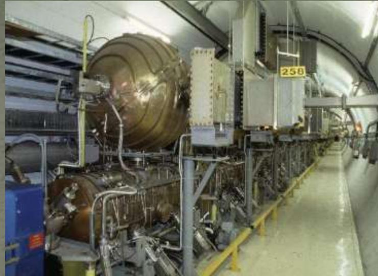
LEP normal-conducting Cu RF cavities,
