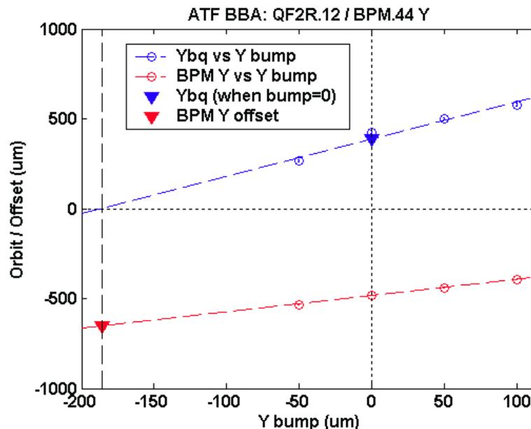
Beam-based alignment in the KEK-ATF damping ring:
