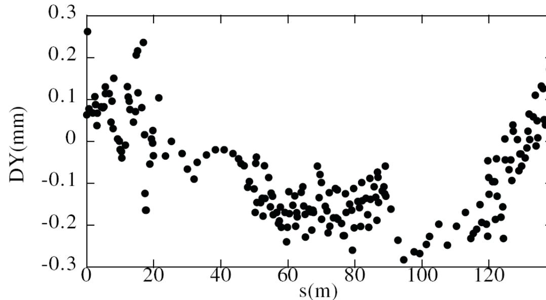
Vertical alignment of the magnets is critical:
