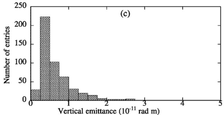
Simulations of emittance tuning in the ATF damping ring.
