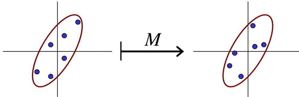
This is not sufficient to determine the beam emittances – though this condition will determine the lattice functions (which can be obtained from the *eigenvectors* of  $\Sigma \cdot S$ ).
